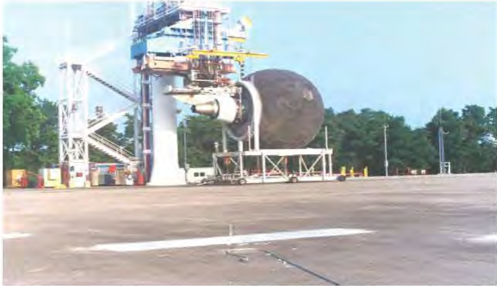
Figure 5.1: Acoustic test bench of a turbofan engine, CFM property
