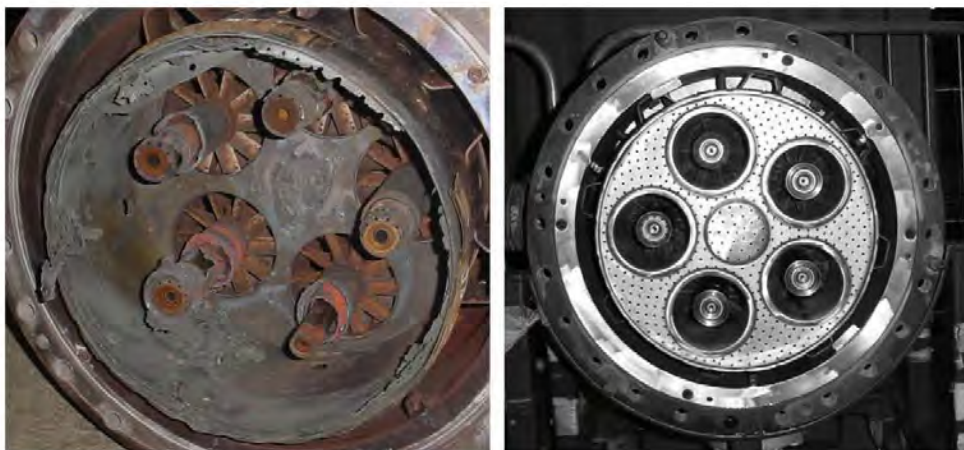
Figure 6.1: Burner assembly damaged by combustion instability (left) and new burner assembly (right) [ Goy et al., 2005 ].
