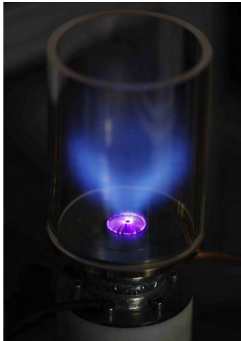
Figure 7.2: Photographic representation of the burner with a lean premixed \text{CH}_4/\text{Air} swirl-stabilized flame (blue) and NRP discharges (purple), from Lacoste et al. [2013a] .
