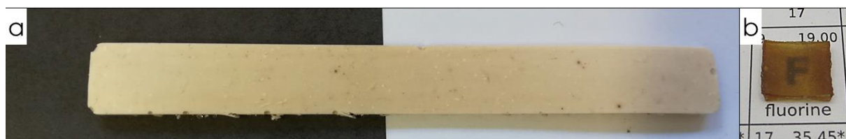
Figure 3. a. Crosslinked material after 8 h at room temperature (ca. 20 °C); and b. after 3 h at 150 °C
