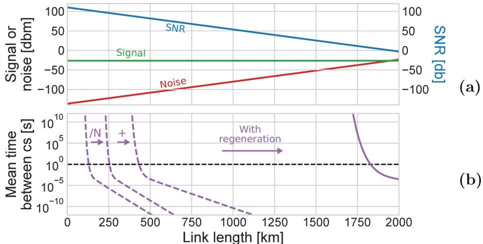
FIGURE 2.10: (a): Signal (green), noise (red), and signal-to-noise ratio (SNR) (blue), at 1 Hz bandwidth, as a function of the length of a fiber link, with repeater laser stations (RLSs) along the link. (b): The corresponding mean time between cycle slips  $\bar{T}$  of the regenerated signal. Results of  $\bar{T}$  shown in figures 2.8 and 2.9 shown in dashed lines.
