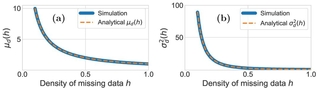
FIGURE 4.4: Monte Carlo simulation of (a): the mean distance  $\mu_d(h)$  and (b): variance on the distance  $\sigma_d^2(h)$  between missing data points for a binomial annihilation operator, as a function of the density of missing data  $h$ . Orange dashed curves show equations 4.3 and 4.4.
