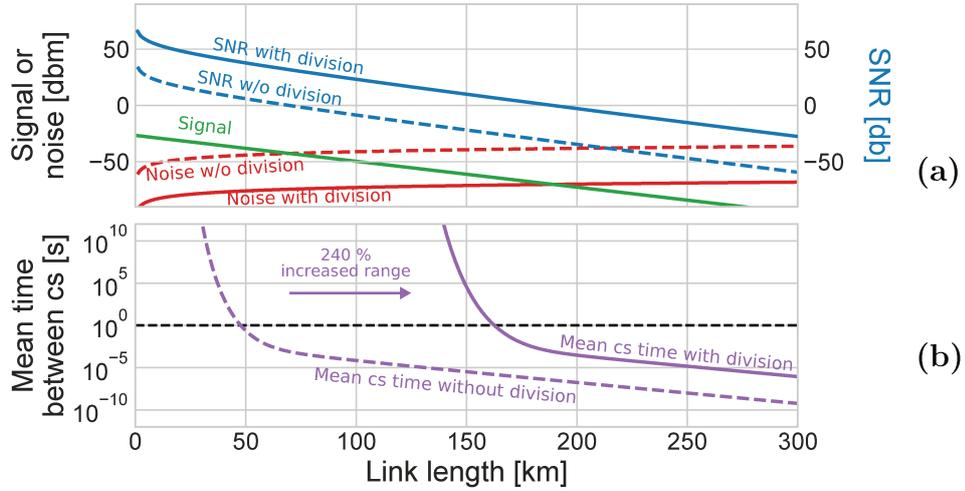
FIGURE 2.8: (a): Signal (green), noise (red), and signal-to-noise ratio (SNR) (blue), in a 1 Hz bandwidth, as a function of the length of a fiber link. (b): Corresponding mean time between cycle slips  $\bar{T}$ , calculated with the SNRs in (a), by equation 2.8. Dashed lines indicate noise, and corresponding SNR and  $\bar{T}$ , without a division factor (according to equation 2.7). Continuous lines corresponds to noise which is divided down (equation 2.9).
