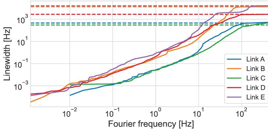
FIGURE 3.5: Linewidth broadening contribution of the 5 links in the REFIMEVE network. Dashed lines show the linewidth contributions as calculated using equation 3.3. Continuous lines show the cumulative linewidth contribution, as calculated using equation 3.6.
