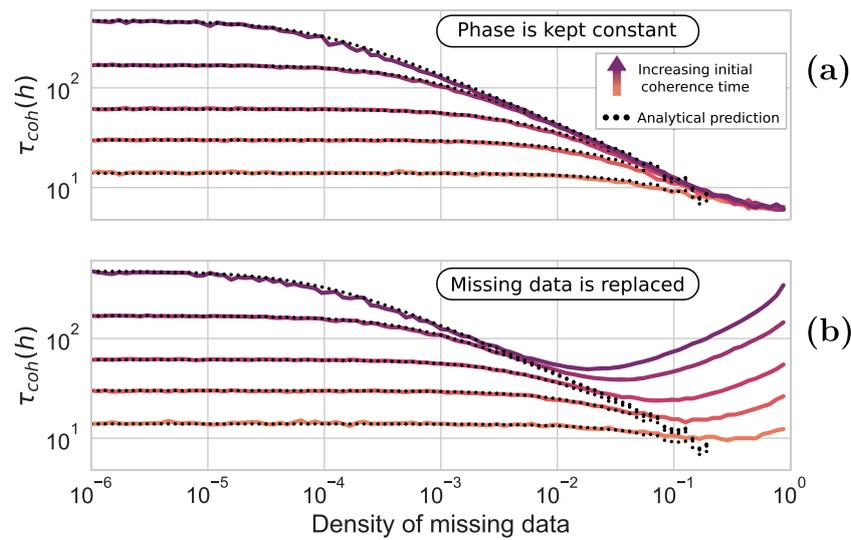
**Figure 10.** Effective coherence time of a simulation of a link as a function of density of missing data. Solid lines indicate the numerically calculated coherence time, with an increasing initial coherence time (increasingly purple). (a) When the phase is kept constant over the missing data, and (b) when missing data is replaced by simulated noise with a similar behavior of that of the link. Equation (7) is shown by black dotted lines.
