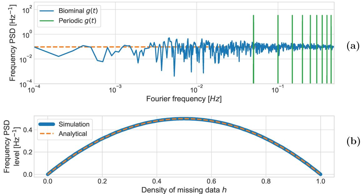
FIGURE 4.6: (a): Spectrum of periodic (green) and binomial (blue) annihilation operators  $g(t)$ , with a density of missing data  $h = 0.05$ . (b): Change in white frequency noise level of the binomial  $g(t)$  as a function of  $h$ . Dashed orange curves in both plots corresponds to equation 4.7.
