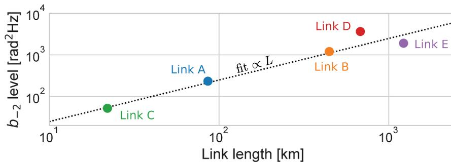
FIGURE 2.7: The level of white frequency noise  $b_{-2}$  for the noise of the first spans of the five links in the REFIMEVE network, as a function of their respective lengths  $L$  (colored dots). The dotted line shows a fit with slope  $\kappa L$ . The links are explained in chapter 2.3.
