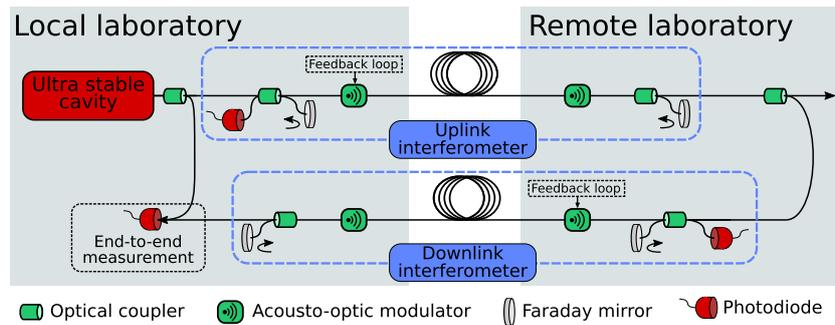
**Figure 1.** Illustration of the active noise compensation scheme (ANC) used for long distance fiber links. The end-to-end measurement is recorded as the beat node between the local ultra-stable cavity and the light disseminated first in the uplink, and afterward in the downlink interferometer.
