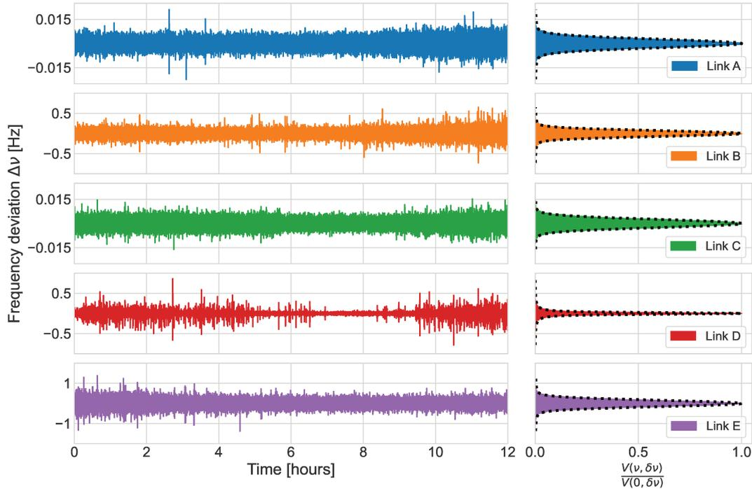
FIGURE 3.8: Frequency fluctuations of the five links over a duration of half a day. The right part shows the distributions of the frequency fluctuations, with black dotted lines corresponding to Voigt fits according to equation 3.15.
