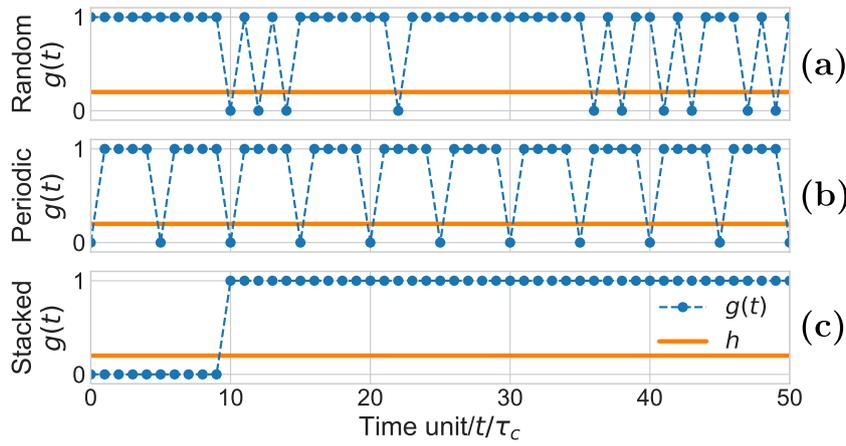
**Figure 7.** Illustration of three different representations of the annihilation operator  $g(t)$ , showing examples of (a) random, (b) periodic, and (c) stacked missing data. The density of missing data,  $h = 0.2 = 20\%$ , is the same in all 3 cases.
