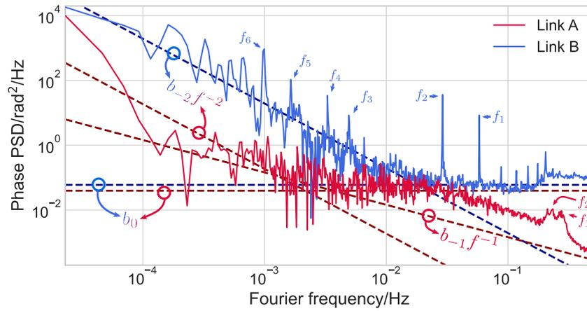
**Figure 3.** PSD of the phase noise, for Link A (red) and Link B (blue), with a linear density of points per decade. The noise coefficients  $b_n$  are indicated from equation (A.3) and are listed in table 1.
