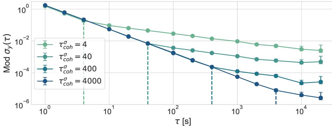
FIGURE 3.10: Illustration of the use of the coherence integration time  $\tau_{\text{coh}}^\sigma$ , defined by equation 3.14, for generating simulated data. The four different stability curves correspond to four different values of  $\tau_{\text{coh}}^\sigma$ . Dashed lines indicate  $\tau_{\text{coh}}^\sigma$  of each respective simulation.
