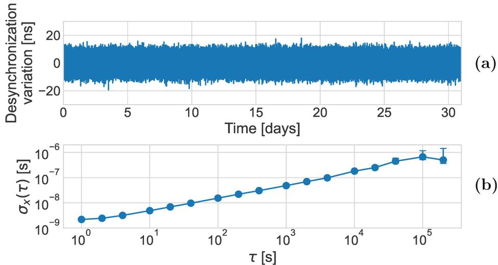
FIGURE 5.11: (a): Variation of the desynchronization of the remote frequency counter in Strasbourg, after the subtraction of the mean value of 0.5 ms. (b): Time deviation (TDEV) of the desynchronization. The desynchronization is calculated from the measurement of an FSK signal as shown in figure 5.10, by equation 5.4.
