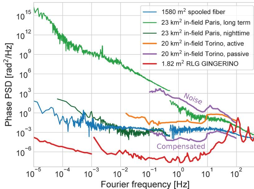
FIGURE 6.7: Comparison between the two configurations in Paris, with an active [100] and passive [19] experiment on a 20 km<sup>2</sup> loop in Torino, Italy, and the 1.82 m<sup>2</sup> ring laser gyroscope (RLG) GINGERINO in Italy [104, 105].
