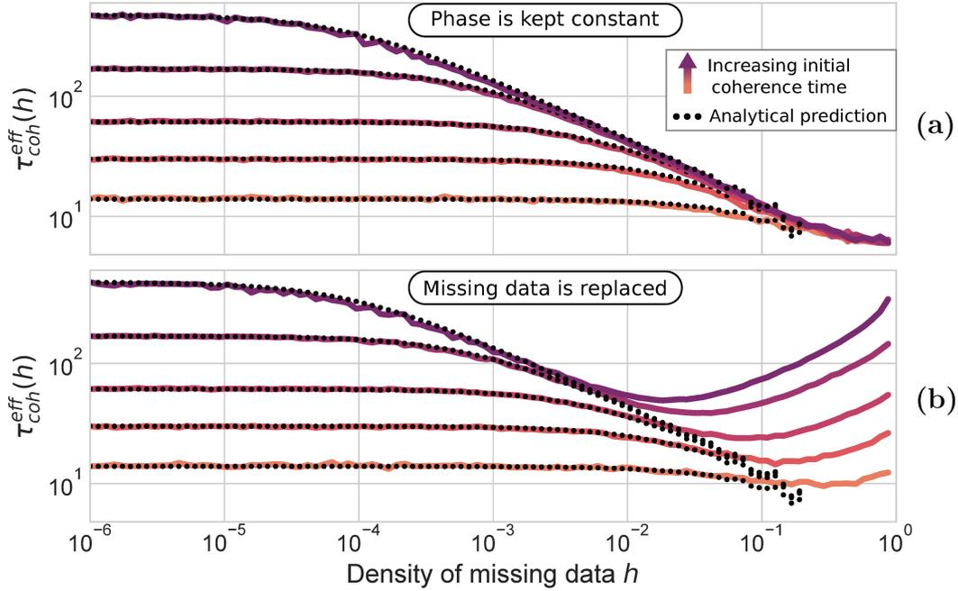
FIGURE 4.9: Effective coherence time of a simulated link  $\tau_{\text{coh}}^{\text{eff}}(h)$  as a function of the density of missing data  $h$ , where (a): the phase is kept constant across the gap left by missing data, and (b): missing data is replaced with simulated noise. Increasingly purple color indicates increasing initial coherence time of the simulation, with no missing data present. Black dotted curves show equation 4.12.
