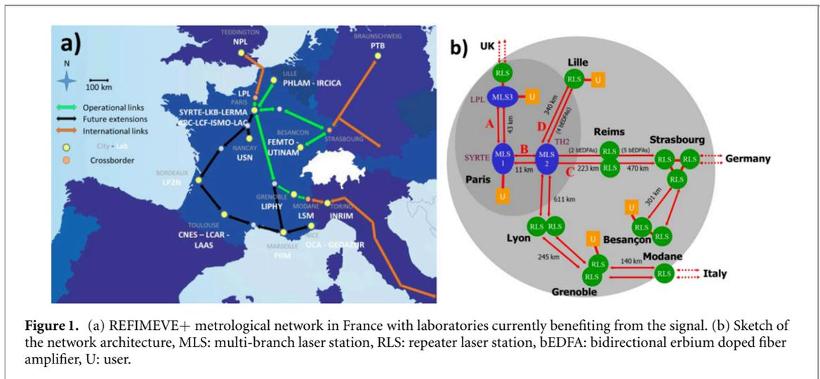
**Figure 1.** (a) REFIMEVE+ metrological network in France with laboratories currently benefiting from the signal. (b) Sketch of the network architecture, MLS: multi-branch laser station, RLS: repeater laser station, bEDFA: bidirectional erbium doped fiber amplifier, U: user.
