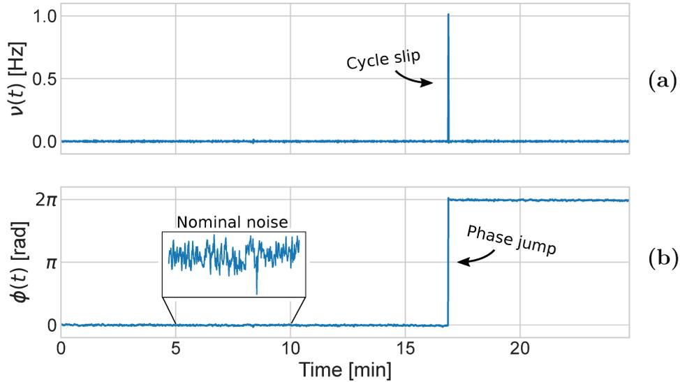
FIGURE 3.2: (a): Frequency fluctuations and (b): phase fluctuations of Link A over a duration of 25 minutes. A cycle slip around the 17<sup>th</sup> minute is highlighted. Insert showing nominal phase fluctuations.
