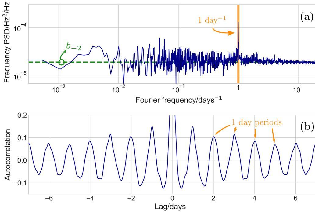
**Figure 11.** (a) Long term frequency PSD and (b) autocorrelation of Link B. The green dashed line shows the  $b_{-2}$  noise parameter from table 1. 1 day fluctuations are noted with orange arrows and writing in both the Fourier frequency (a) and time (b) domain.
