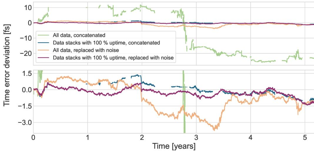
FIGURE 4.14: Phase evolution of Link B over 5 years, calculated in 4 different ways: from all data stacks (green), only data stacks with 100 % uptime (blue), all data stacks where missing data is replaced with simulated noise (light brown), and only data stacks with 100 % uptime where missing data is replaced with simulated noise (purple). Bottom plot is a zoom of the top plot.
