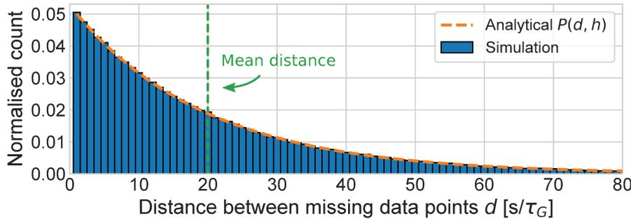
FIGURE 4.3: Monte Carlo simulation of the distance between missing data points for a binomial annihilation operator, with a density of missing data  $h = 0.05$ . The orange dashed curve shows equation 4.2, and the mean distance is indicated by the vertical green line.
