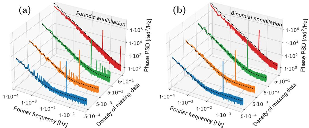
FIGURE 4.7: Aliasing effects of a white phase noise signal with a strong periodic modulation, with an increasing amount of missing data. (a): Periodically spaced missing data, and (b): binomially spaced missing data.
