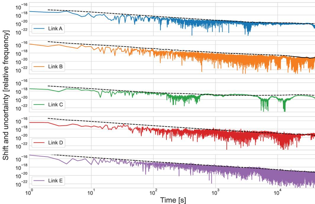
FIGURE 3.9: Cumulative relative frequency shift of the five links in the network of the frequency data presented over half a day in figure 3.8. The black dashed line shows the uncertainty of the shift at a given timescale.
