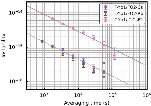
FIG. 5. Instabilities of the ratios between IT-Yb1 and FO2-Cs, FO2-Rb and IT-CsF2 as overlapping Allan deviation. The solid gray line represents the white noise contribution of IT-CsF2 ( $3.2 \times 10^{-13}$  at 1 s for this shorter measurement); the dashed gray line represents the short-term instability of FO2-Rb and FO2-Cs ( $4.3 \times 10^{-14}$  at 1 s).
