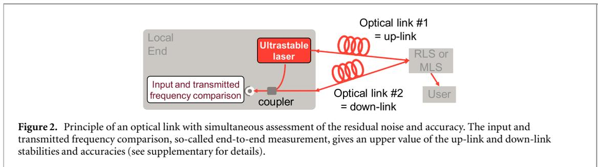
**Figure 2.** Principle of an optical link with simultaneous assessment of the residual noise and accuracy. The input and transmitted frequency comparison, so-called end-to-end measurement, gives an upper value of the up-link and down-link stabilities and accuracies (see supplementary for details).
