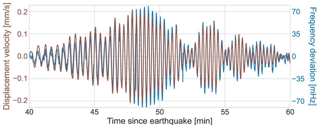
FIGURE 6.11: Overlap of the detection of an earthquake by Link A (blue), and the East component of a nearby seismometer (brown), over the duration of 20 minutes. The time trace of Link A and the seismometer are both a cut-out of the traces shown in figure 6.10.
