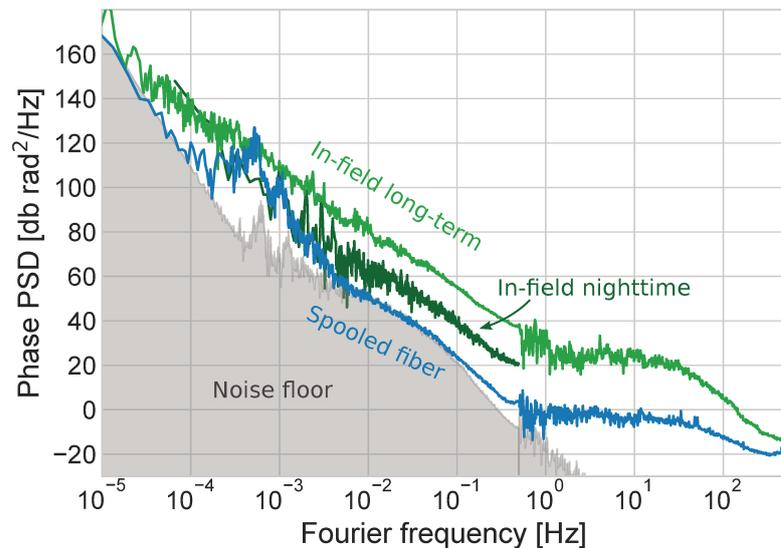
FIGURE 6.5: Sum of the two beat notes, according to equation 6.3, of the two configurations: the 25 km,  $1580 \text{ m}^2$  fiber spool (blue), and the 28 km,  $23 \text{ km}^2$  in-field loop (green). Light-green shows the long-term behavior of the in-field configuration, and dark green shows the behavior during the night.
