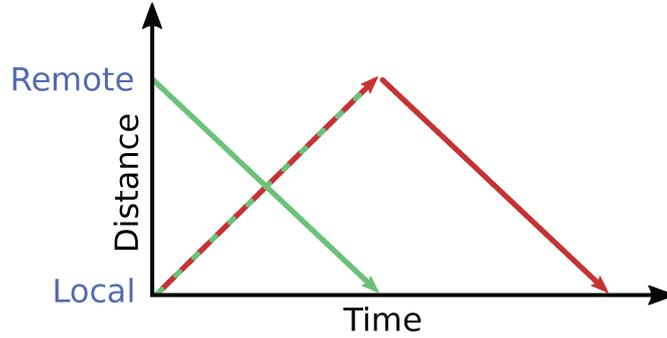
FIGURE 2.3: Illustrative comparison between travel times of signals in a fiber, in an active compensation scheme (red and red/green arrows), and a two-way scheme (green and red/green arrows). Plot derived from Claudio Calosso.
