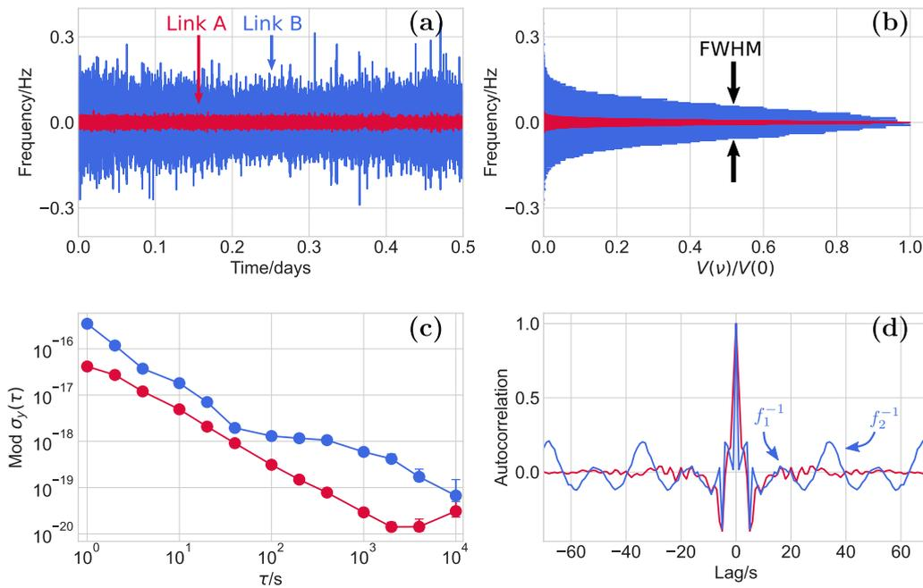
**Figure 2.** Behavior of the noise of Link A (red) and Link B (blue) for half a day of measurement time, with a gate time of  $\tau_G = 1$  s. (a) Frequency fluctuations. (b) Normalized distribution of frequency fluctuations. (c) MDEV of the fractional frequency fluctuations. (d) Auto-correlation of the frequency fluctuations. Arrows point out two of the periodic perturbations in Link B.
