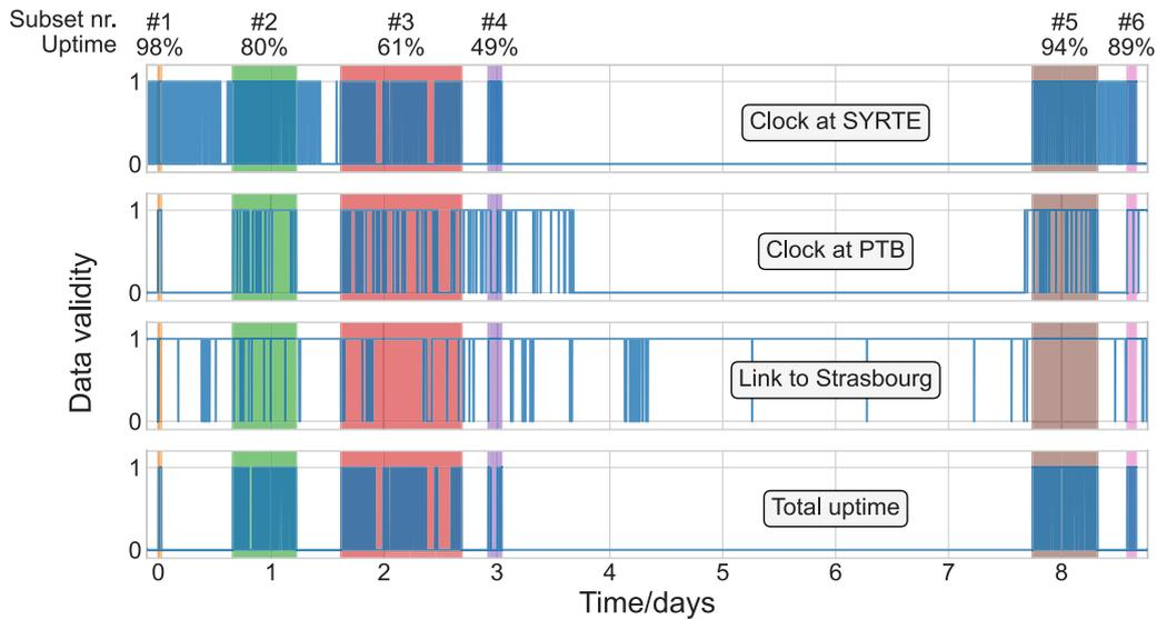
**Figure 13.** Illustration of the operation time of the two clocks, Link B, which is used in their comparison, as well as the total uptime of the comparison. From the total uptime, 6 subsets are chosen and analyzed individually.
