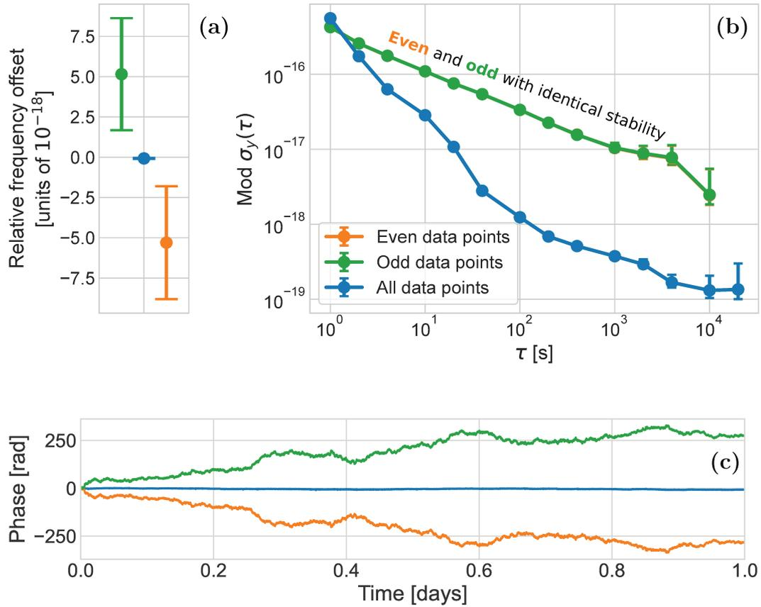
FIGURE 4.1: (a): Uncertainty, (b): modified Allan deviation, and (c): phase evolution of one full day of Link B, using the full data set (blue), or only using the even (orange) or odd (green) points.
