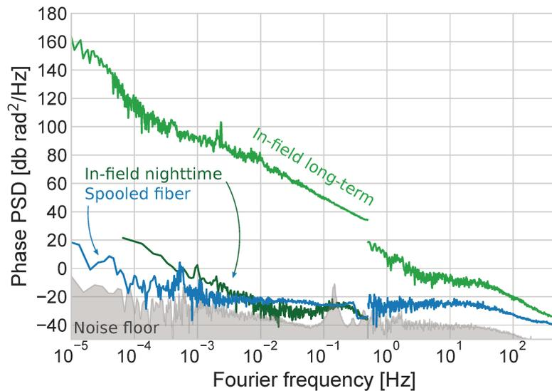
FIGURE 6.6: Difference between the two beat notes, according to equation 6.2, of the two configurations: the 25 km, 1580 m<sup>2</sup> fiber spool (blue), and the 28 km, 23 km<sup>2</sup> in-field loop (green). Light-green shows the long-term behavior of the in-field configuration, and dark green shows the behavior during the night.
