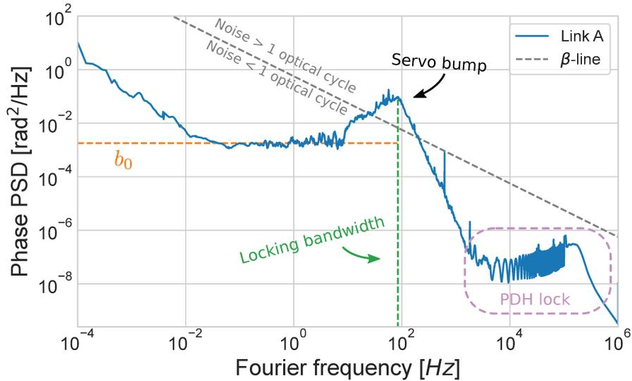
FIGURE 3.3: Phase power spectral density (PSD) of Link A (blue). Lines represent the level of white phase noise  $b_0$  (orange), its locking bandwidth (green), and the  $\beta$ -line (gray). The pink box highlights the Pound–Drever–Hall (PDH) lock limit.
