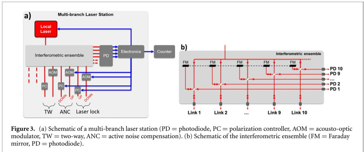
**Figure 3.** (a) Schematic of a multi-branch laser station (PD = photodiode, PC = polarization controller, AOM = acousto-optic modulator, TW = two-way, ANC = active noise compensation). (b) Schematic of the interferometric ensemble (FM = Faraday mirror, PD = photodiode).
