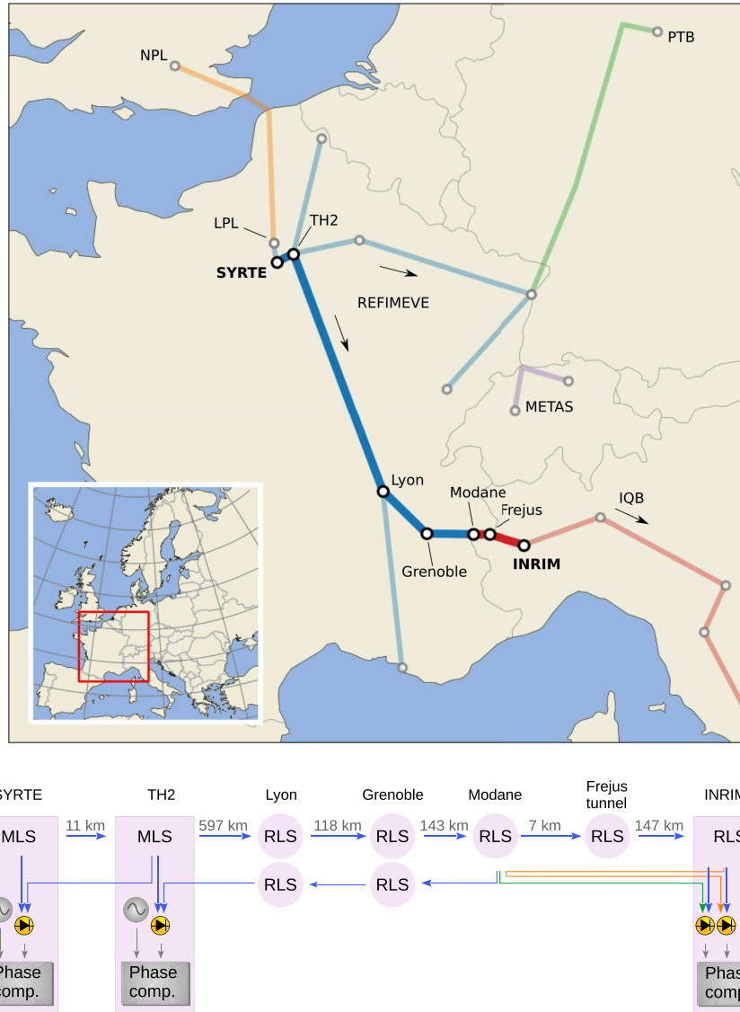
FIG. 1. Geographical layout of the infrastructure, with the link between SYRTE, Paris (France) and INRIM, Torino (Italy) characterized in this work highlighted as a thick line. The map also shows the other branches of the REFIMEVE network in blue and the Italian Quantum Backbone (IQB) in red. Cross-border connections of this infrastructure to the National Metrology Institutes NPL in the UK and PTB in Germany are indicated in orange and green. Repeater laser stations (RLS or MLS) and link terminals are represented with open circles. (b) The scheme used for the link characterization: blue paths indicate phase-stabilized links on the two fibers. At SYRTE, local reference light is sent to a photodiode together with the light disseminated through the loop SYRTE-TH2-SYRTE and phase compared to a local rf reference, to evaluate the overall uncertainty of the SYRTE-TH2-SYRTE link (similarly for the path to Modane). The green arrow represents a free-running link whose noise is removed offline. This is detected by heterodyning local radiation at INRIM with light traveling the path INRIM-Modane-INRIM (orange line). The Modane-INRIM link is evaluated by comparing light disseminated through the two fibers.
