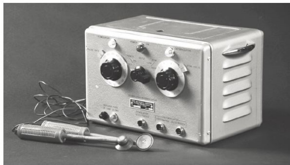
Figure 1-2 The original pacemaker designed by Hopps (Photo courtesy of the National Research Council of Canada)
