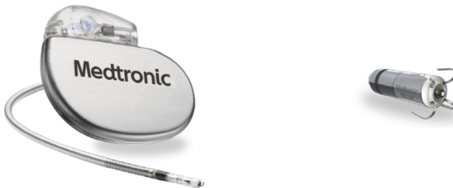
Figure 1-5 Pacemakers a) Traditional single-chamber pacemaker and lead; b) Leadless pacemaker, Micra Medtronics
