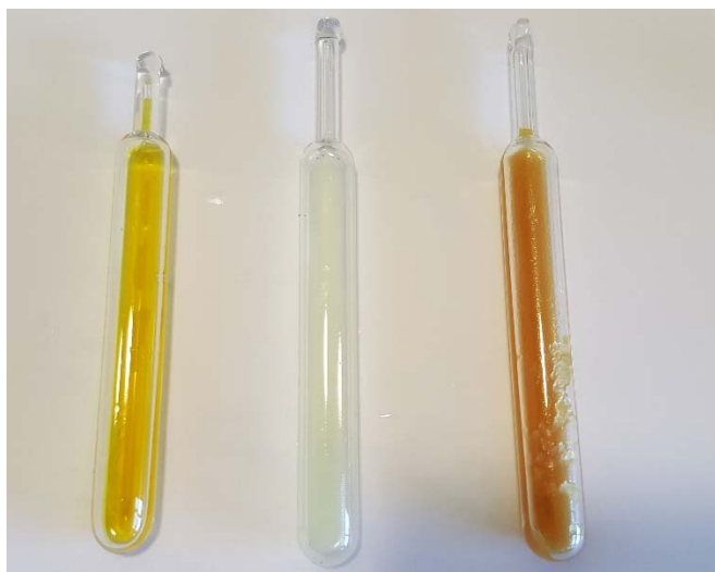
Figure 17. Carius tubes containing PVDF after 24 h of polymerization activated thermally (left), with visible light (center) and UV irradiation (right).
