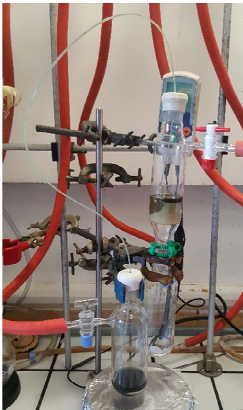
Figure 2. Picture of the filtration system used for the K[Mn(CO)_5] solution to remove the residual NaK.
