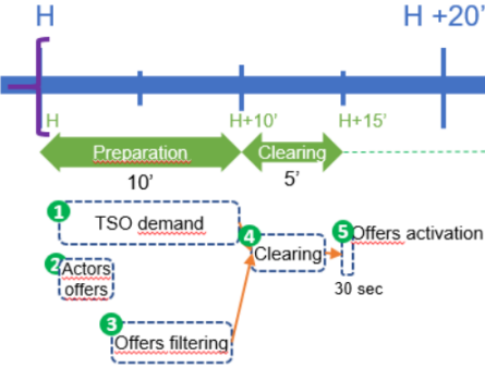
Figure 3- 3 Example of possible TERRE process with clearing every 15 minutes, zoom on first 20 minutes
