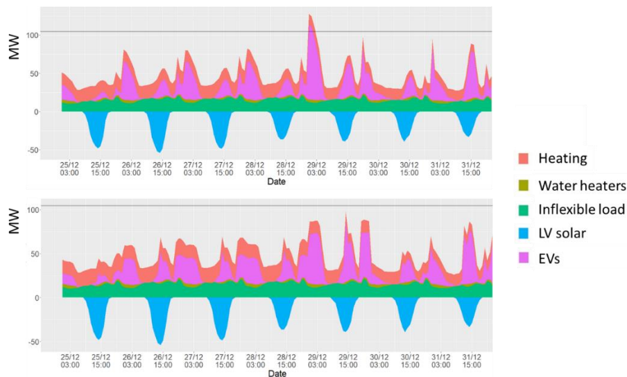
Figure Appendix - 2 Consumption curve for a substation before and after POS filtering
