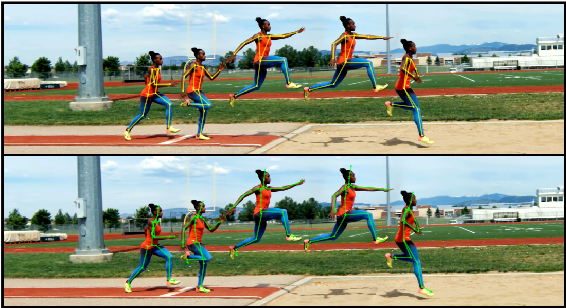
Figure 3.1 – Illustration of our method applied to human pose estimation: the yellow 12-joint skeletons (top) depicts poses estimated by AlphaPose [192] at different timestamps. Our approach completes and upsamples joints in a spatially and temporally consistent way to enrich estimated pose sequences, and yields the corresponding green 28-joint skeletons (bottom). In both images, the background has been stitched from a video with a smaller field of view and five images of the jumper at different frames have been overlaid as foreground.
