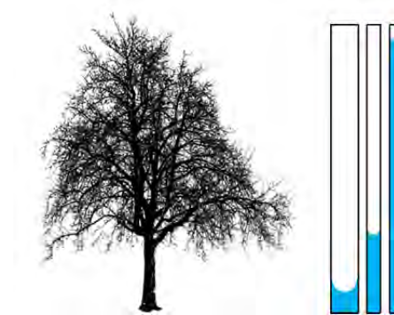
Figure 1-1 Schematic illustration of capillary transport on the example of tree capillaries: large trees need very small capillaries to supply the treetop with liquid.
