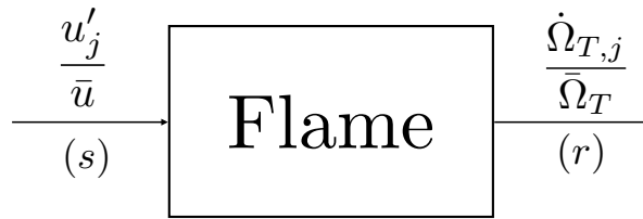
Figure 8.2: The flame viewed as a dynamical system: its input is an upstream acoustic velocity while its output is an unsteady heat release rate.
