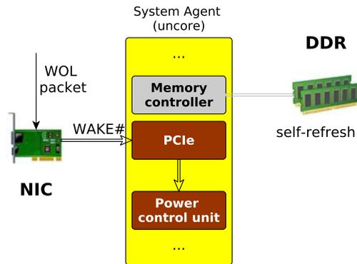
Figure 3.6: The state of the uncore subsystem in  $S_3$ . The memory controller is powered off and the memory banks are in self-refresh mode. However, some components are powered-on and ready for the wake-on-LAN. Following a WOL magic packet, the NIC sends a WAKE signal to the power management controller which perform the system wake-up.
