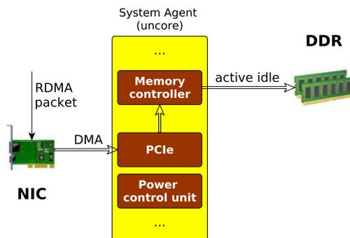
Figure 3.7: The state of the uncore subsystem in  $S_z$ . The memory controller, the memory banks and the entire PCIe circuitry are now active. In this state, the RDMA NIC is able to address the entire memory.
