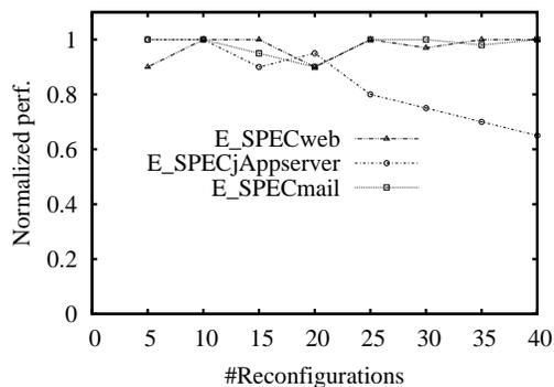
Figure 2.15: Impact of performing several reconfiguration operations. Both E\_SPECmail and E\_SPECweb are relatively little impacted by the multiplication of reconfiguration operations. In contrast, E\_SPECjAppserver’s performance starts to degenerate after about 20 reconfigurations. The degradation comes from the synchronization of the data base tier, which requires a little downtime of the application.
