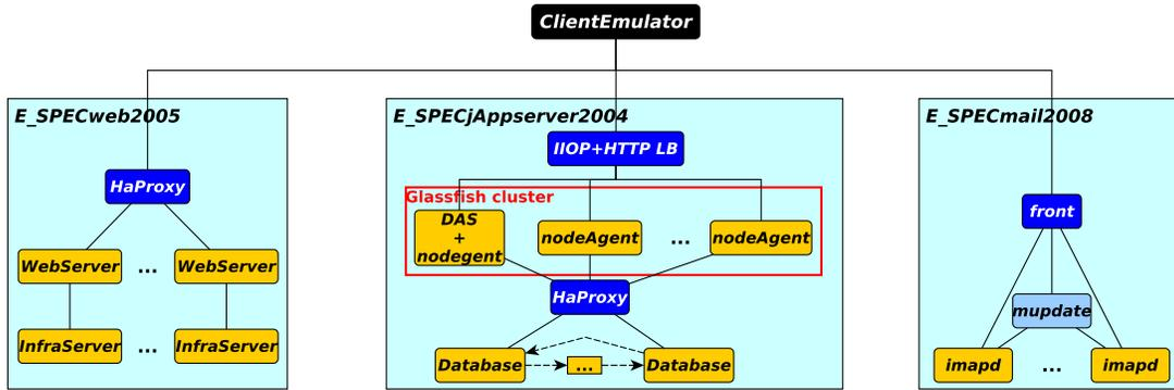
Figure 2.7: Architecture of E\_SPECvirt.
