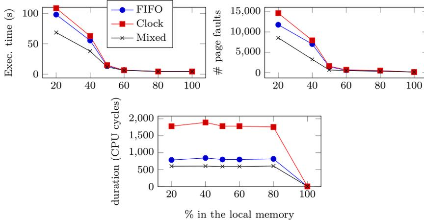
Figure 4.2: Comparison of three replacement policies (FIFO, Clock, and Mixed) for *RAM Ext.* (top) The micro-benchmark execution time, (middle) # page faults and (bottom) time taken by the policy to perform a page fault. Mixed is the best policy.
