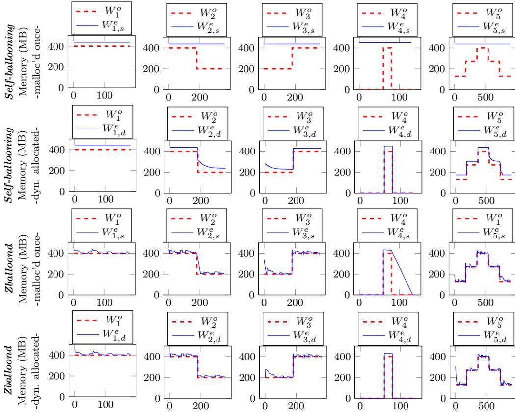
Figure 5.5: Evaluation results of *self-ballooning* and *Zballoond* with synthetic workloads. The original workload is noted  $W_i^o$  while the actual estimated WSSs are noted  $W_{ij}^e$ . "j" is s (the static implementation) or d (the dynamic implementation).
