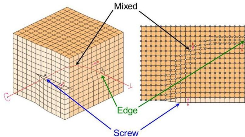
Figure 1. 9: Image of mixed dislocations in an atomic lattice [50].
