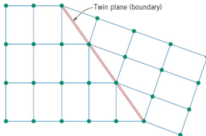
*Figure 1. 11: Schematic of twin plane [53].*
