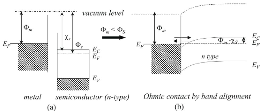
Figure 3.7: Energy band diagram for a metal-semiconductor (n-type) contact, in the case  $\Phi_m < \Phi_s$  before (a) and after (b) they are brought into contact. In this case, ohmic contact formation occurs by band alignment [8].
