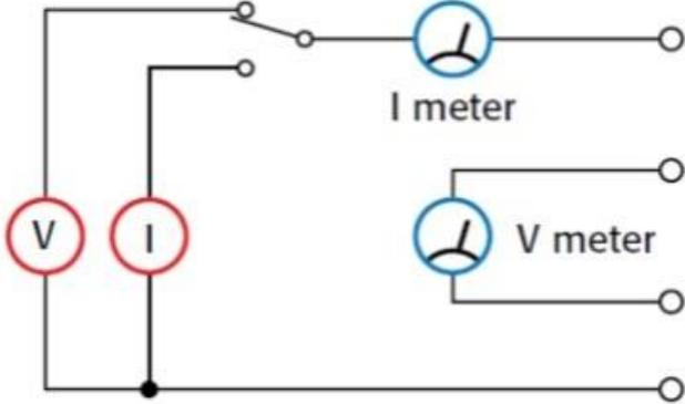
Figure 3. 1: Basic SMU instrument topology [29].
