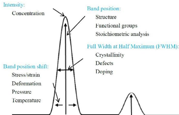
Figure 2. 4: Typical Information from material with Raman spectroscopy [16].
