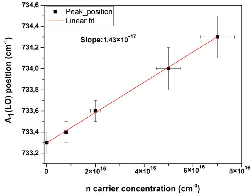
Figure 5. 7: Zoom in the light doping region  $n < 10^{17} \text{ cm}^{-3}$  with a linear approximation fit. The error bars of the carrier concentration have been set based on 10% of the initial Si concentration for each sample.
