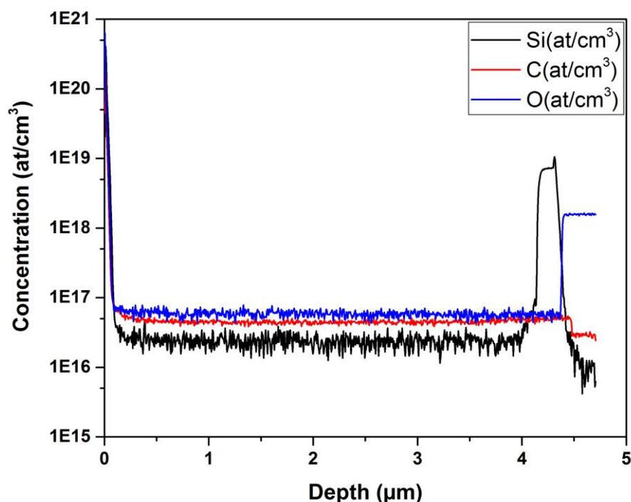
*Figure 6. 4: SIMS results on Epi02 sample. The black curve highlights presence of Si dopants (main dopant). The red and the blue curves represent the background impurities in the sample respectively. This result can also be applied to Epi03 samples because they have been grown on the same way with the same instruments.*
