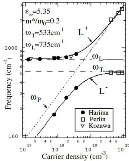
Figure 2. 7: LOPC mode vs carrier concentration for  $n > 10^{17} \text{cm}^{-3}$ .
