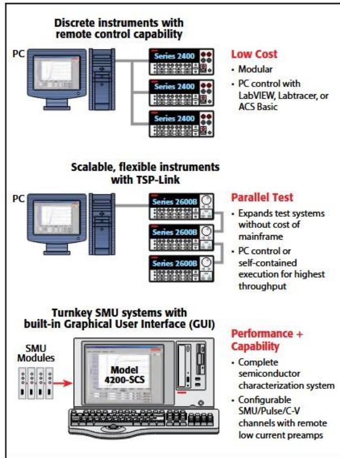
Figure 3.2: Examples of I-V characterization solutions [30].
