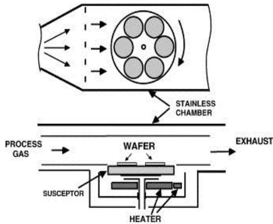
*Figure 1. 3: MOCVD reactor set up for GaN growth [12].*
