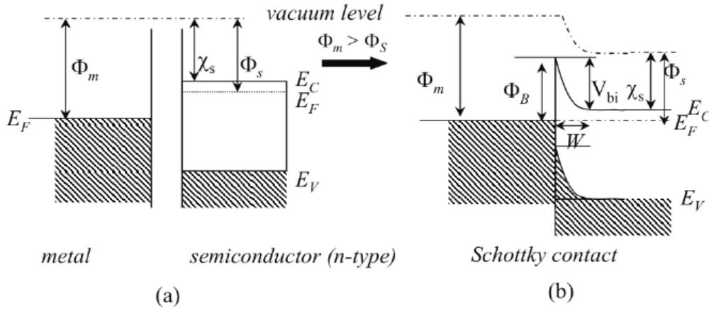
Figure 3.2: Energy band diagram for a metal-semiconductor (n-type) contact, in the case  $\Phi_m > \Phi_s$  before (a) and after (b) they are brought into contact, showing the formation of a rectifying contact with a Schottky barrier height  $\Phi_B$  [8].
