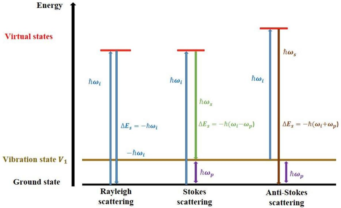
Figure 2. 1: Jablonski diagram for Rayleigh and Raman (Stokes and anti-Stokes) scattering [4].  $\hbar\omega_i$  is the incident energy,  $\hbar\omega_s$  is the scattered energy and  $\hbar\omega_p$  is the phonon energy.
