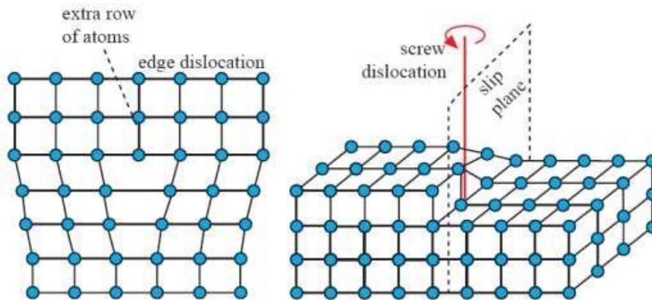
*Figure 1. 8: Schematic diagrams of an edge and screw dislocation in an atomic lattice [38].*
