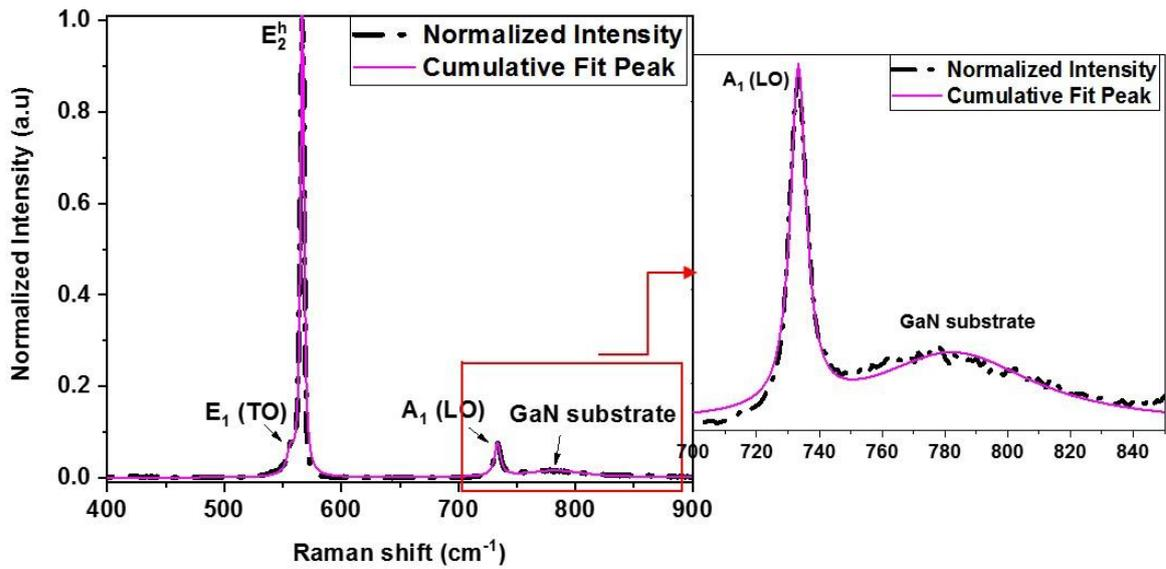
Figure 5. 3:  $A_1$  (LO) fittings for  $A_1$  (LO) Raman maps extraction. The fittings have been performed by taking account of the GaN substrate signal in order to subtract its quantitative influence.
