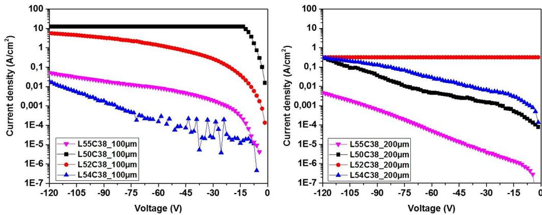
Figure 7. 6: Reverse  $I(V)$  semi-log plots of  $100\mu\text{m}$  (left) and  $200\mu\text{m}$  (right) diodes of Epi03 drift layer.
