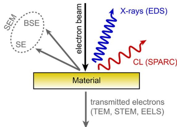
Figure 2. 9: Material analysis based on the incident electron beam.
