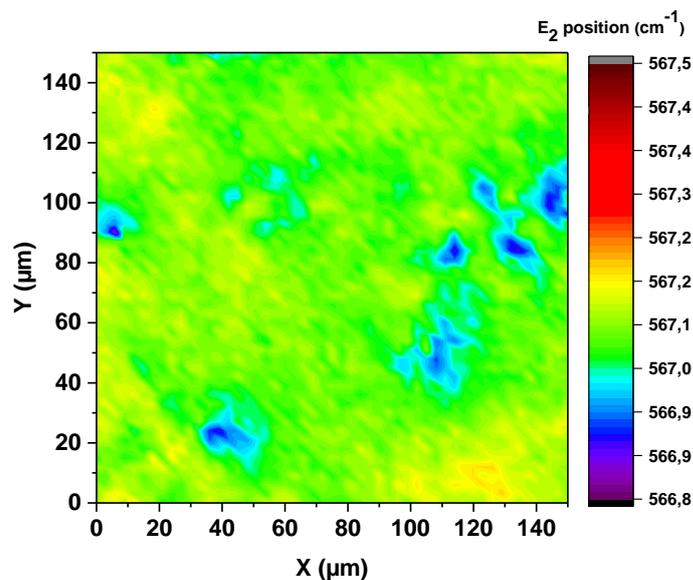
Figure 4. 5:  $E_2^h$  position map example of one substrate. The blue spots may be some dislocations during substrate growth
