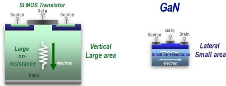
Figure 1.12: GaN based vertical and lateral devices respectively [96].
