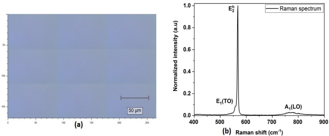
*Figure 4. 2: (a) Raman microscope image of the GaN substrate surface. (b) Raman spectrum from the cartography.*
