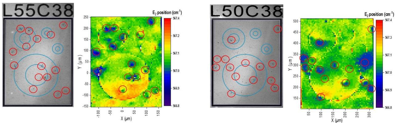
Figure 6. 8:  $E_2$  position 2D Raman map alongside their corresponding cathodo-luminescence images (scale bar: 100  $\mu\text{m}$ ) performed on the diodes for Epi03 (column C38).
