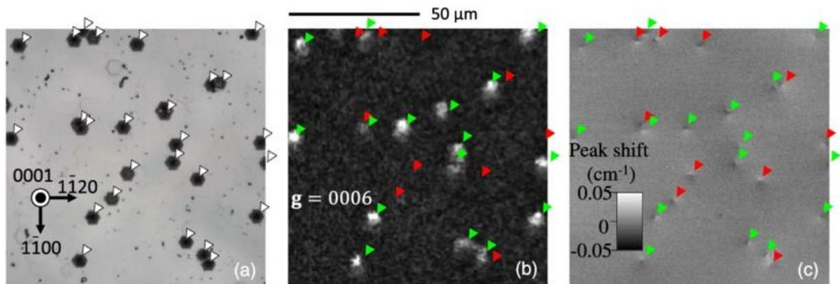
*Figure 2. 8: (Color online)  $100 \times 100 \mu\text{m}^2$  area images of (a) etch pits, (b) X-ray topography taken along the  $g=0006$ , and (c) Raman mapping of the  $E_2$  (high) peak shift. The location of the etch pit are illustrated by dotted white triangles. The red and green triangles correspond to the TED and TMD, respectively.*
