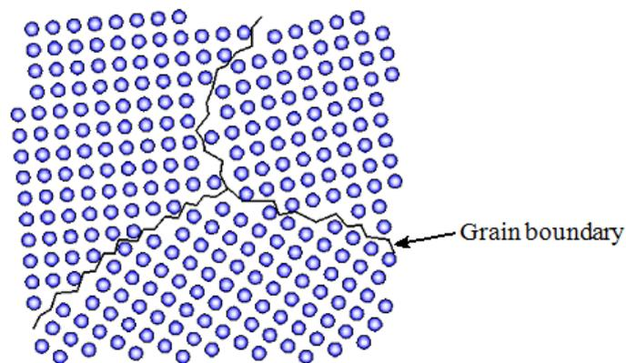
Figure 1. 10: Illustration of planar defects in atomic lattice [51].
