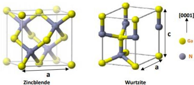
Figure 1. 5: Zinc blende and Wurtzite GaN polytypes [19].
