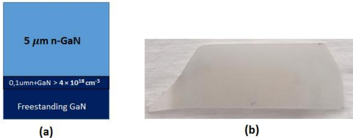
*Figure 5. 1: (a) Schematic cross section image of the homo-epitaxial sample with a highly doped (n+ doping) GaN buffer layer (0.1 μm thickness) on a freestanding GaN substrate. (b) Image of the n doped GaN epilayer.*
