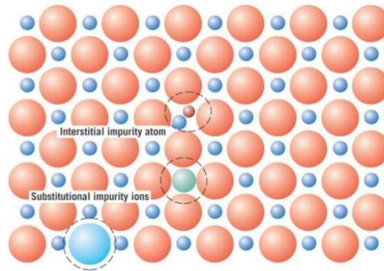
*Figure 1. 7: Illustration of common type of point defects [32].*
