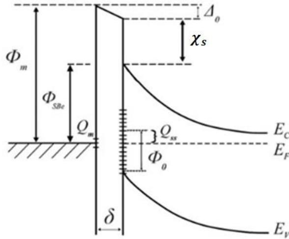
Figure 3.3: Energy band diagram of a contact between a metal and an n-type semiconductor with interface states in the band gap at the semiconductor surface. The charge  $Q_{ss}$  in the interface states creates a dipole over a distance  $d$  that lowers the barrier height by  $\Delta_0$  [4].
