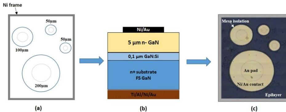
*Figure 3.8: (a) Cross section of the mask design before metallization. (b) Cross section of the vertical GaN Schottky diodes. (c) Optical image of the diodes after metallization. Scale bar for the image in figure c is 100  $\mu\text{m}$ .*
