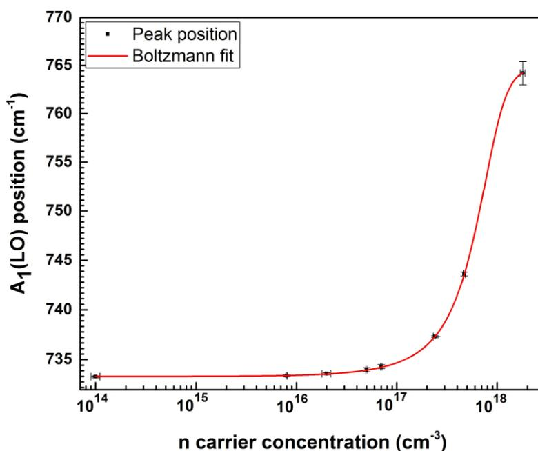
*Figure 5. 6: Calibration of the  $A_1(\text{LO})$  position as function of the  $n$ -doping concentration in log scale. The square dark dots are the experimental data and the red line is the fitting Boltzmann evolution growth curve.*
