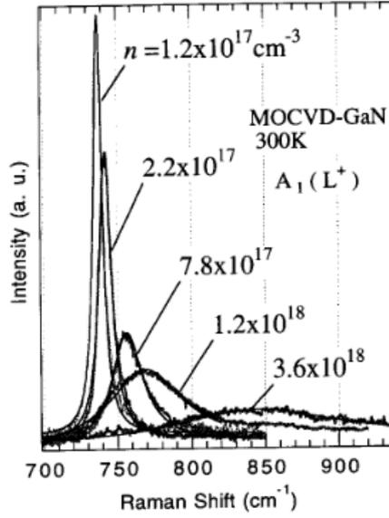
Figure 2. 6: LOPC mode evolution vs carrier concentration.
