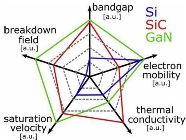
Figure 1. 1: Comparison of the relevant material properties for Si, SiC and GaN power electronics [4].
