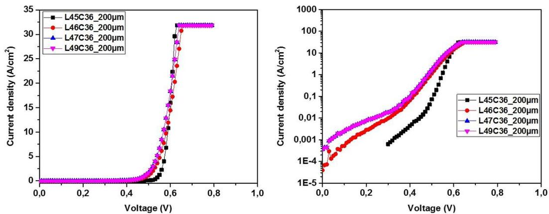
Figure 7. 2: Forwards  $I (V)$  plots of  $200\mu\text{m}$  diodes of Epi02 drift layer. Left hand side is the linear scale plot and right hand side is the semi-log scale plot. The constant current density is due to the limitation of the compliance value.
