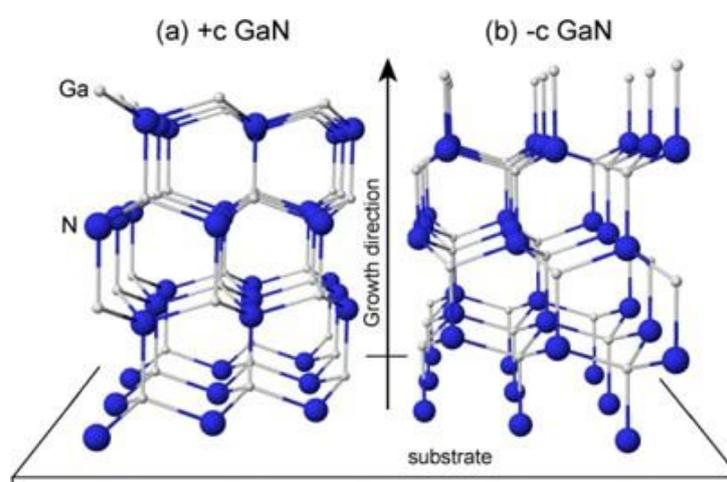
*Figure 1. 6: Schematic illustration of GaN wurtzite crystal structure exhibiting the polarity along the c axis. The small and large spheres indicate Ga and N, respectively. GaN with Ga-face (+c) polarity on left side and GaN with N-face (-c) polarity on right side. When the direction of the three bonds of the III element is towards the substrate, the polar structure*
