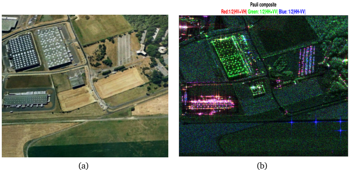
Figure A.1: (a) Google Maps optical image, Brétigny (France), May 2004. (b) Pauli color composite Ramses Brétigny data.
