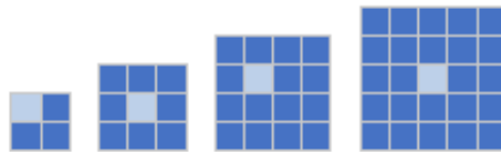
Figure 2.2: Illustration of the analysis parameter “bin size” with a value of 2, 3, 4, and 5, respectively. The analyzed pixel is shown in light blue, and its neighbors are shown in deep blue.
