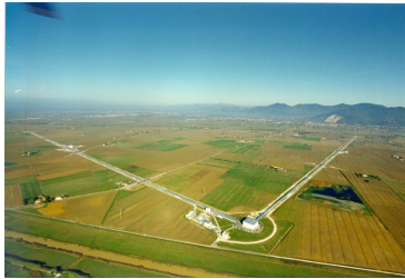
Figure 2.3: Aerial view of Virgo the European gravitational wave detector. Virgo detector has two arms of 3 kilometers.
