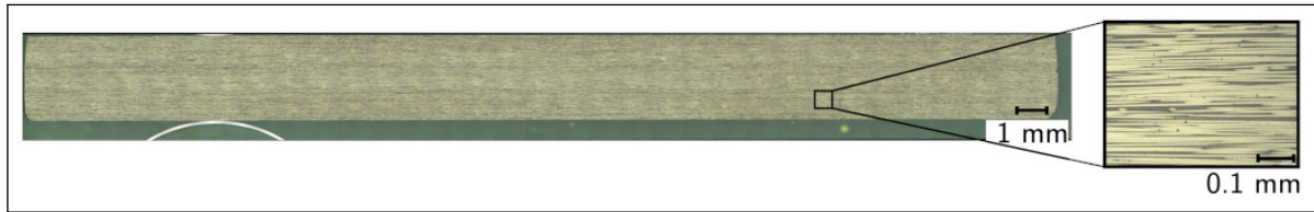
Figure 4.1: Micrograph (cross section parallel to the fibers main axis) of the consolidated samples before deconsolidation tests (objective magnification \times 200 and resolution 1.55^2 \mu\text{m}^2/\text{pixel} ). The initial porosity content is not measurable.
