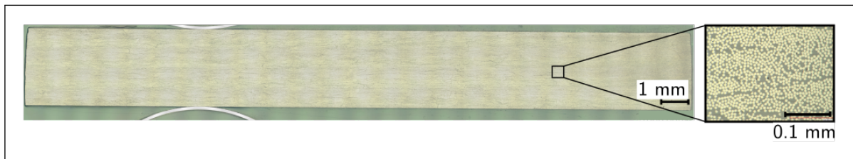
Figure 5.5: Micrograph of the consolidated samples before deconsolidation tests (objective magnification \times 200 and resolution 1.55^2 \mu\text{m}^2/\text{pixel} ). The initial porosity content is not measurable.
