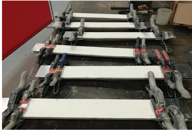
Figure 3- 130 : Preparation of a TRM specimen for the direct tensile test: gluing of aluminum tabs.
