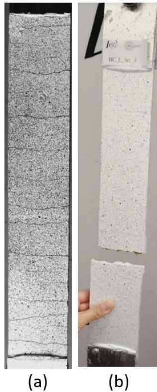
Figure 4- 182 : Failure mode B recorded in all the HC-L series, a) multiple stress behavior during stage II, and b) the rupture of the yarns at the end of stage III.
