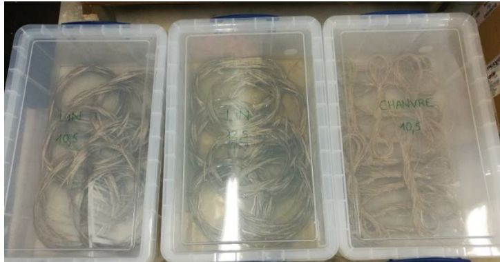
Figure 3- 79 : Accelerated aging of yarns at T=23^{\circ}\text{C} .
