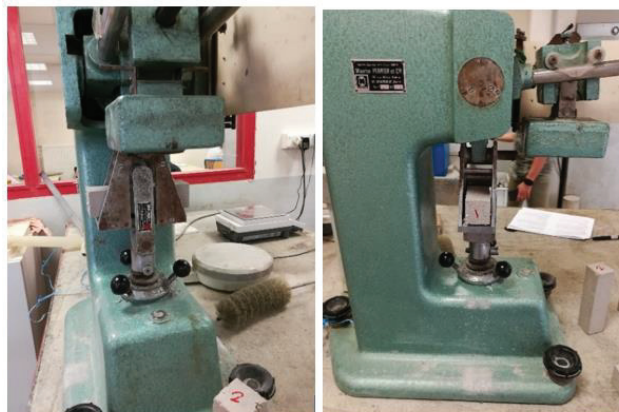
Figure 2- 54 : 3-point bending test setup on a 40 mm x 40 mm x 160 mm matrix specimen.
