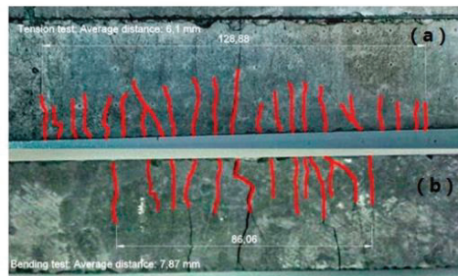
Figure 1- 42 : cracking maps of two composites from the same plate tested under tensile (a) and bending (b) tests [146].
