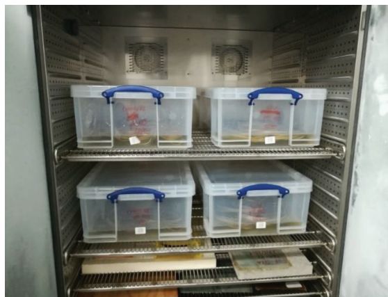
Figure 3- 80 : Accelerated aging of yarns at T=40^{\circ}\text{C} or 60^{\circ}\text{C} .
