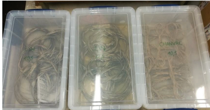
Figure 3- 79 : Accelerated aging of yarns at T=23^{\circ}\text{C} .
