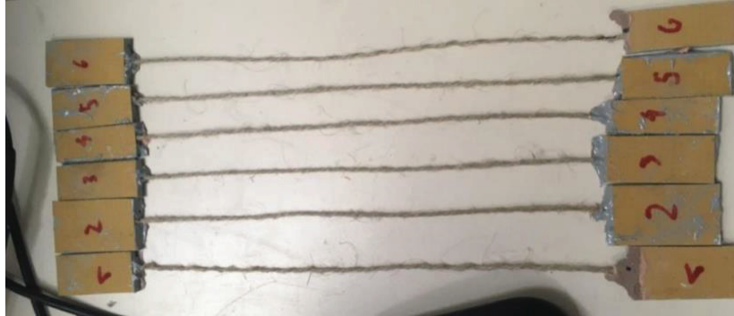
Figure 2- 73 : Fiberglass composite tabs glued to the both ends of the bio-resin-coated hemp yarns.
