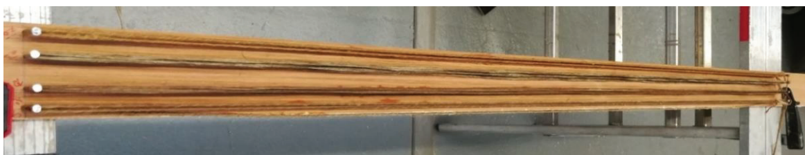
Figure 3- 81 : Drying of the hemp and flax yarns after removal from the aging solutions.
