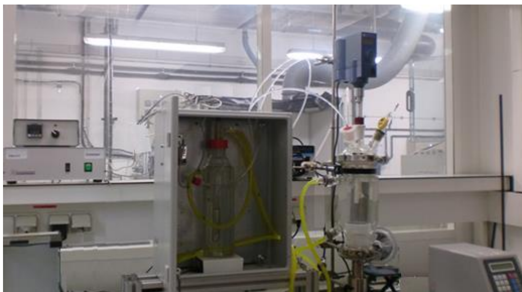
Figure 2.24. Schematic drawing and photograph of the sono-photochemical reactor system
