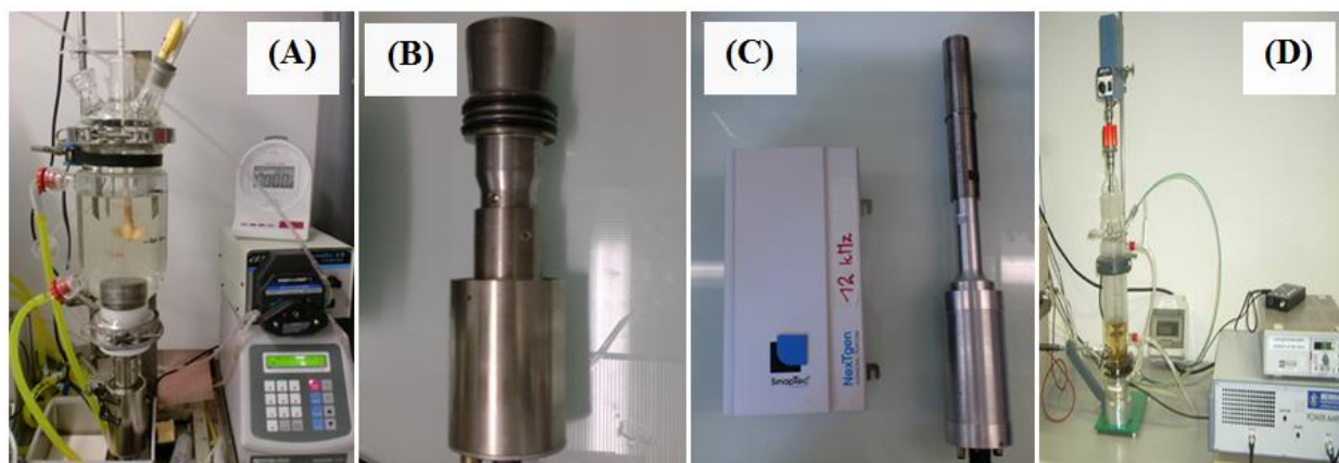
Figure 2.18. Ultrasonic equipment 1 mounted in sono-reactor (A), ultrasonic probe of equipment 1 (B), ultrasonic equipment 2 (C), and sono-reactor with ultrasonic equipment 3 (D)
