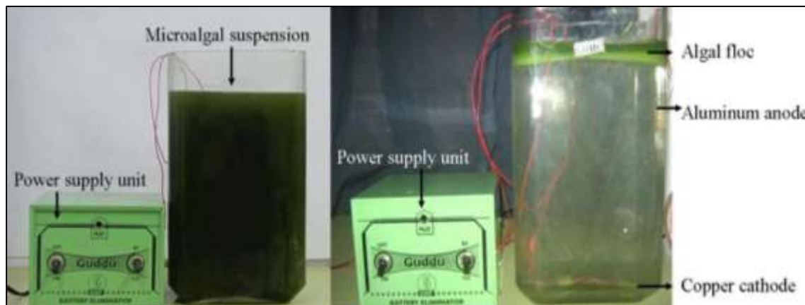
Figure 16- A laboratory model showing electro-coagulation–flocculation of microalgae [103].
