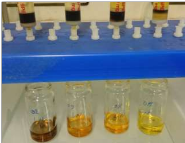
Figure 37- Solid Phase Extraction (SPE) technique showing the partitioning of lipids to three classes neutral lipids, glycolipids and phospholipid.
