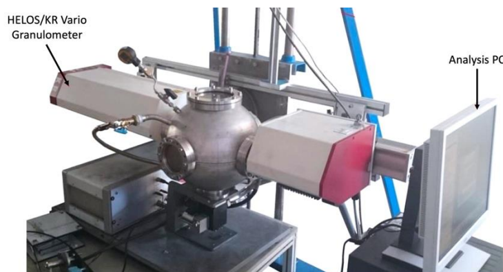
Figure III-6: DSD analysis experimental set-up in the 20 L open sphere - adapted from Murillo (2016)
