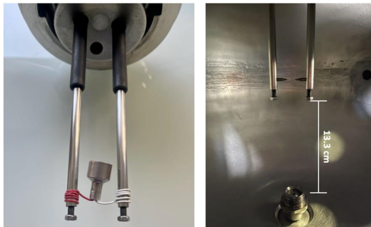
Figure III-9: Employed ignition sources - left: 100 J chemical ignitors (Sobbe GmbH), right: spark ignitors mounted in the 20 L sphere
