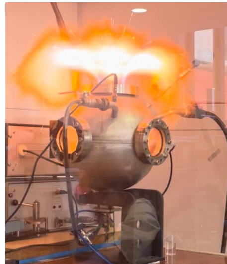
Figure VI-8: Ethanol mist explosion in the vented 20 L sphere
