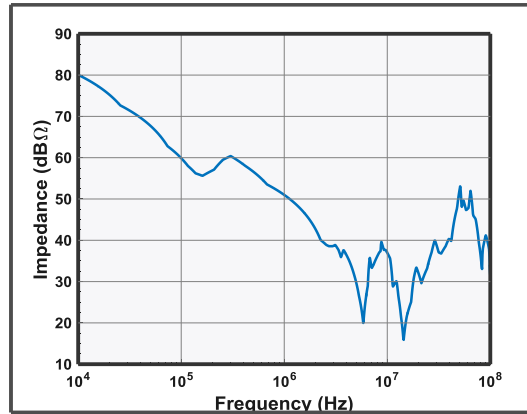
Figure 4.9 : Common mode impedance of the load used in the present work (Hypothesis)
