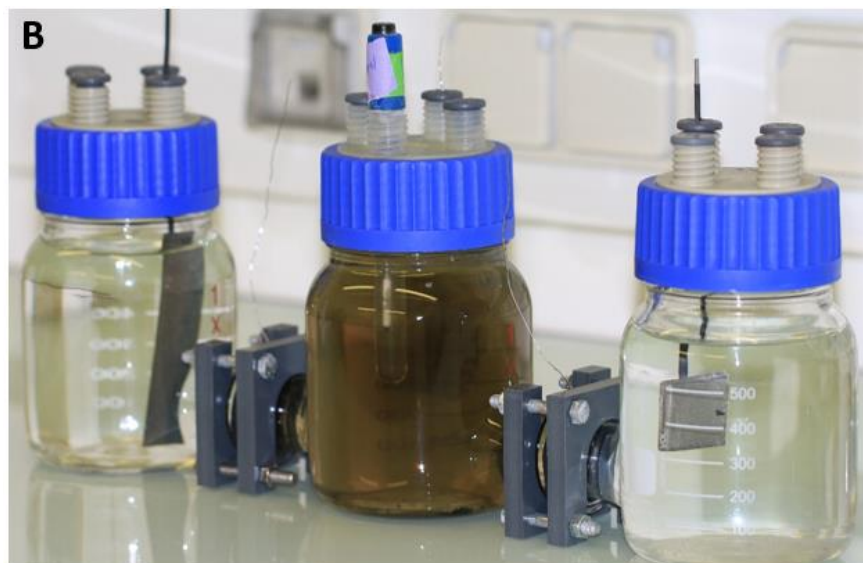
Figure 1: A) Schematic and B) picture of the electrochemical device with garden compost leachate in the central compartment and Medium 2 in the two end-compartments.
