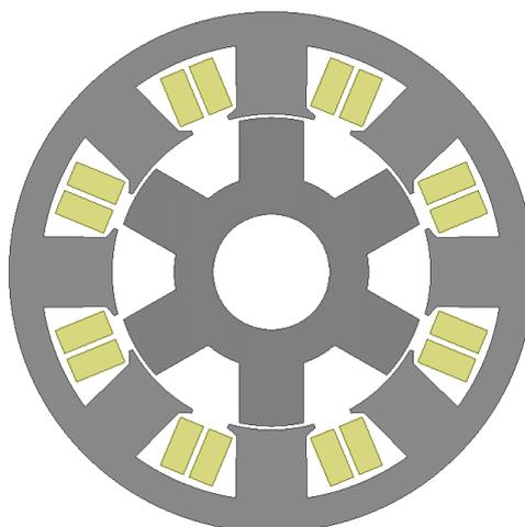
Figure 1. 5: Example of a switched reluctance machine
