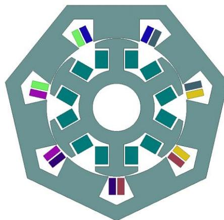
Figure 3. 8: Structure in 2D of the optimal WRSM
