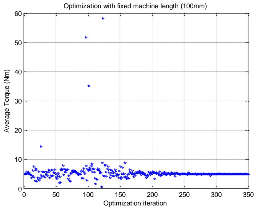
Figure 3. 14: Average torque in Optimization with  $L = 100\text{mm}$
