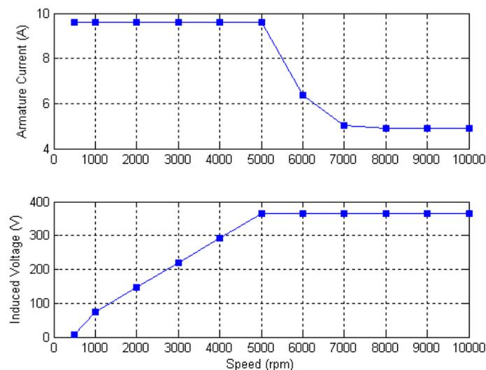
Figure 2. 26: Armature current and voltage of SM-PMSM
