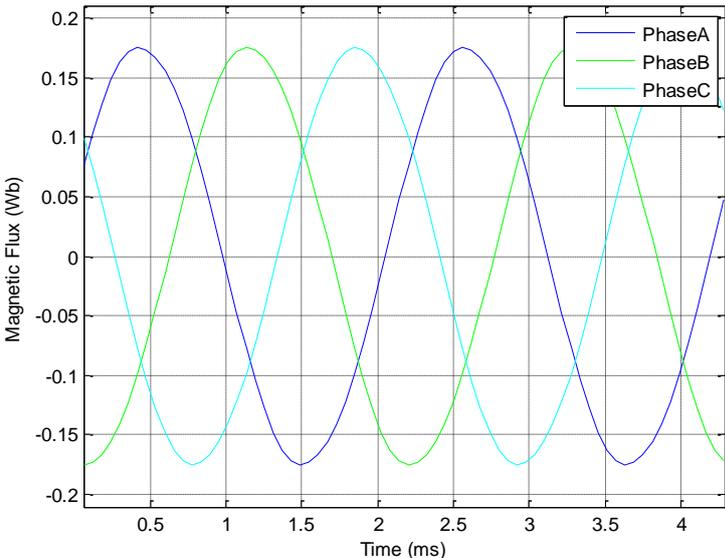
Figure 2: Magnetic flux of the SM-PMSM
