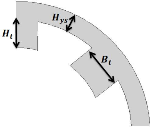
Figure 3. 1: The cylindrical stator variables
