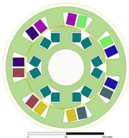
Figure 2. 37: Cylindrical based WRSM
