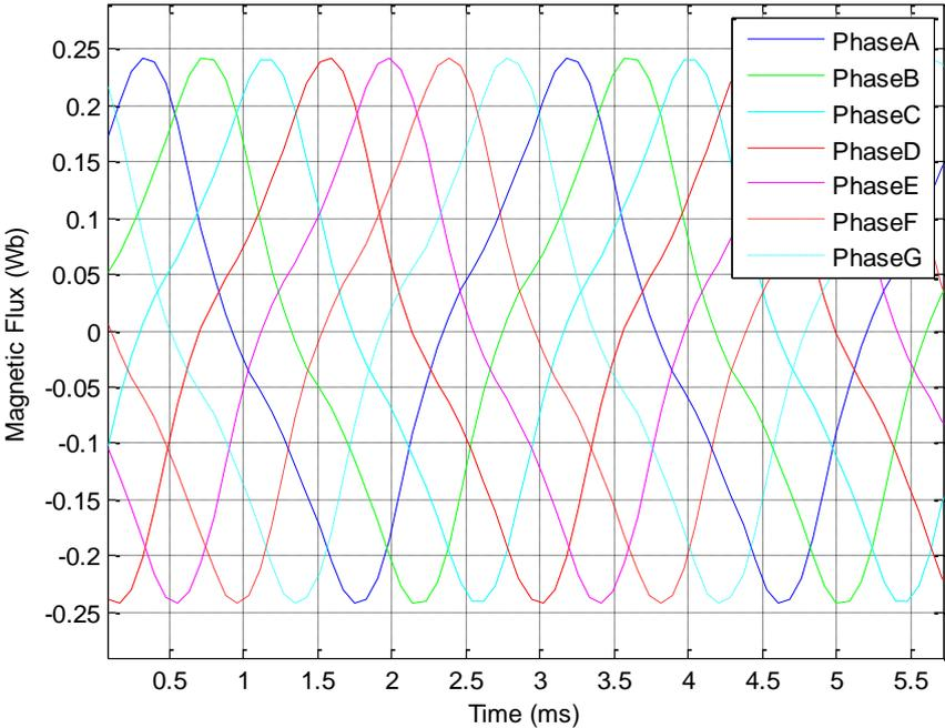
Figure 8: Magnetic flux of the designed WRSM
