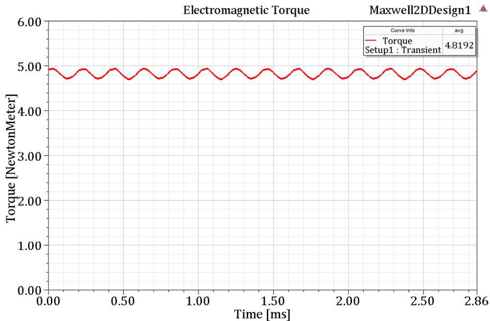
Figure 4. 3: Electromagnetic torque obtained by 2D ANSYS Maxwell 15.1
