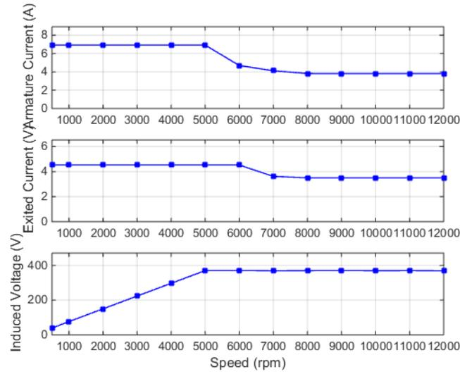
Figure 2. 29: Armature/field currents and voltage of the WRSM
