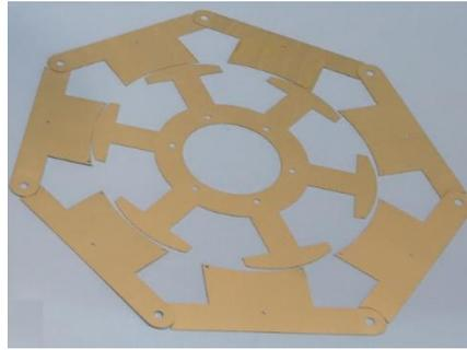
Figure 4. 23: Segmented stator core and rotor core
