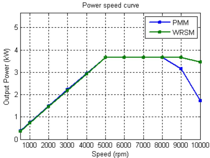
Figure 2. 34: Power vs. speed of the SM-PMSM and WRSM
