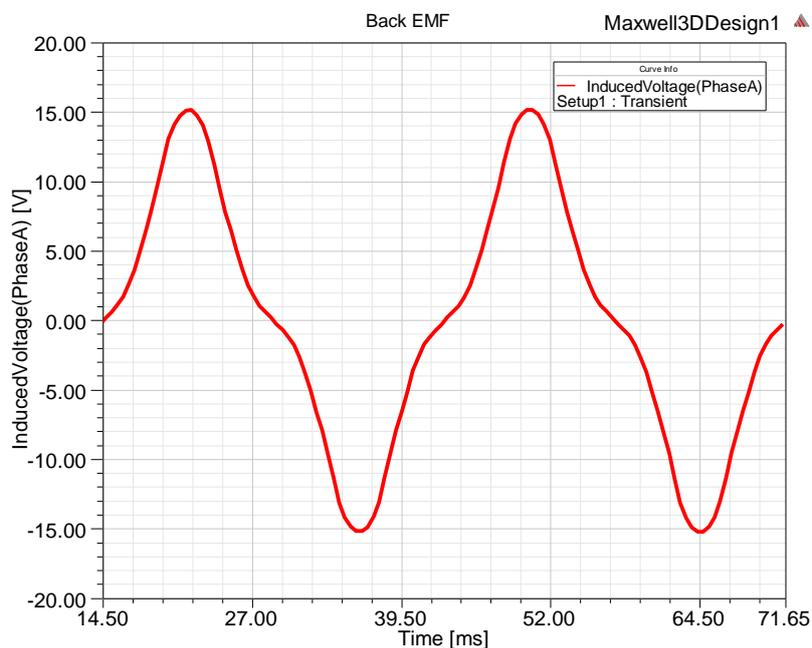
Figure 4. 30: EMF waveform by 3D FE analysis
