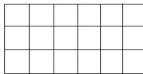
Figure 4. 9: Structured grid
