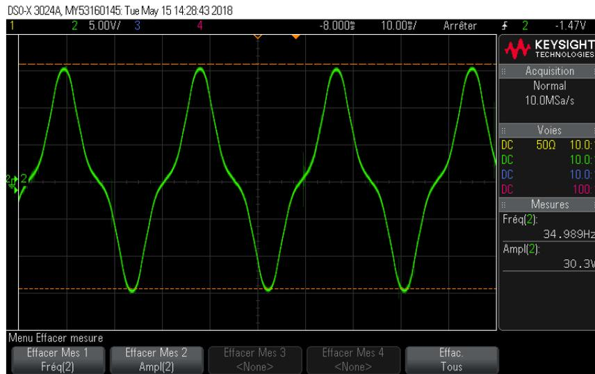
Figure 4. 29: EMF waveform in Oscilloscope
