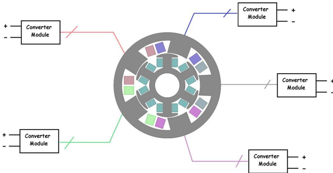
Figure 1. 11: Integrated machine and power supply concept
