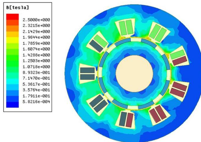
Figure 2. 19: Stator and rotor induction of the SM-PMSM
