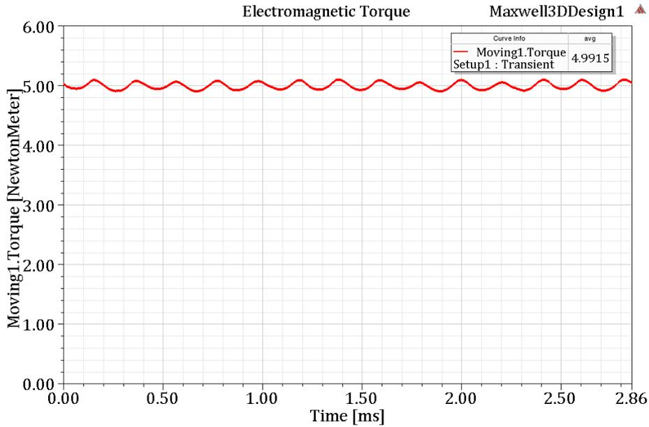
Figure 4. 6: Electromagnetic torque analyzed by 3D ANSYS Maxwell 15.1
