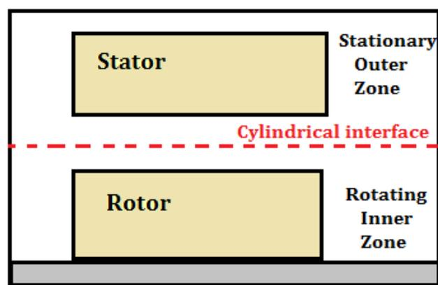
Figure 4. 18: MRF interface of the simplified model
