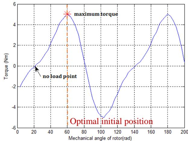
Figure 2. 10: Static torque vs. mechanical rotor angle
