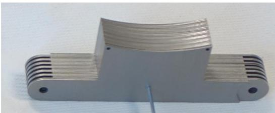
Figure 4. 21: One segment of the stator core
