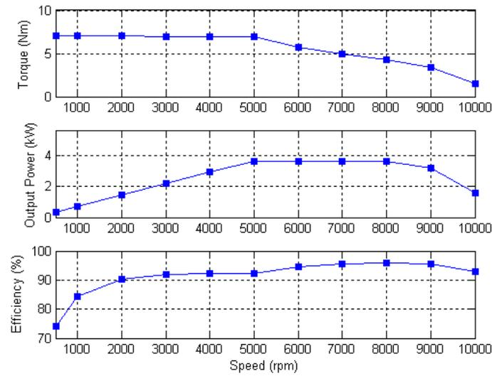
Figure 2.27: Torque power and efficiency of SM-PMSM
