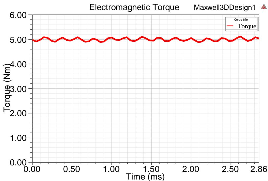
Figure 4. 2: 3D electromagnetic torque of the rectified WRSM
