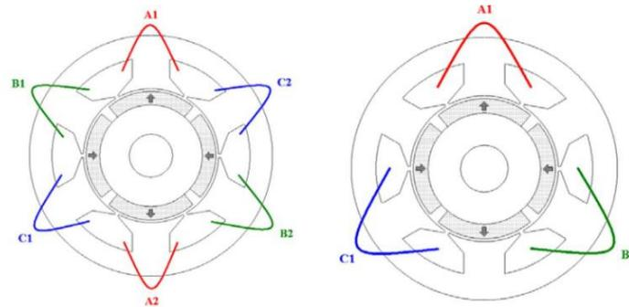
Figure 2. 1: Double layer and single layer windings [59]
