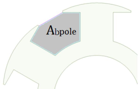
Figure 2. 24: Area between two rotor poles
