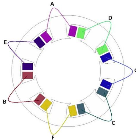
Figure 2. 7: Winding layout of 7-phase/7-slot/6-pole machine
