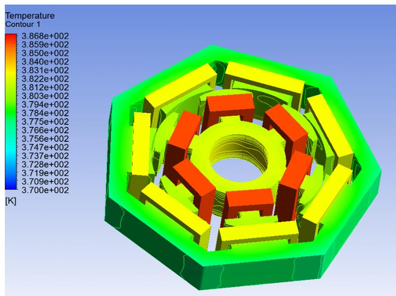
Figure 4. 19: Temperature distribution of the WRSM
