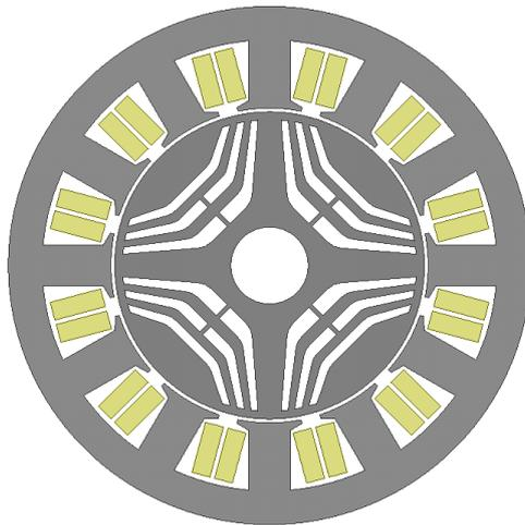
Figure 1. 6: Example of a synchronous reluctance machine
