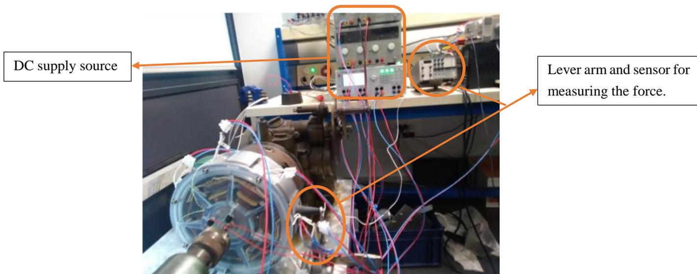
Figure 4. 32: Experimental set-up for testing static torque without converters
