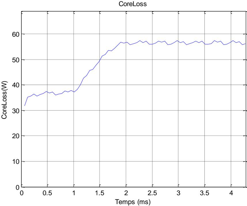
Figure 5: Core losses of the SM-PMSM
