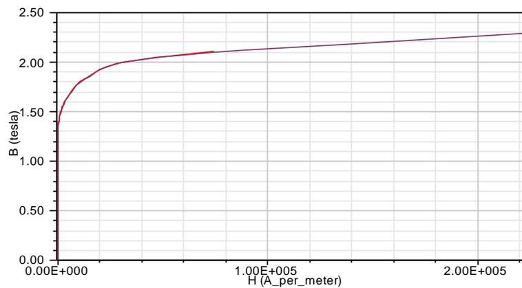
Figure 2. 18:  $B(H)$  curve of DW310-35 material
