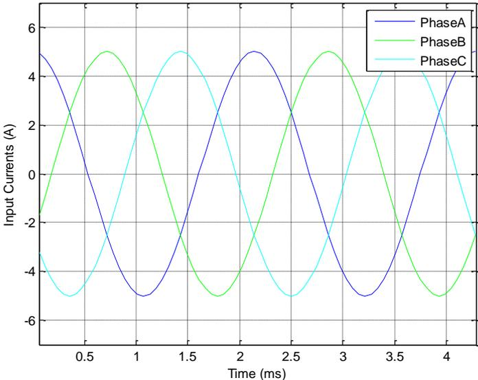
Figure 1: 3-phase sinusoidal input currents for SM-PMSM
