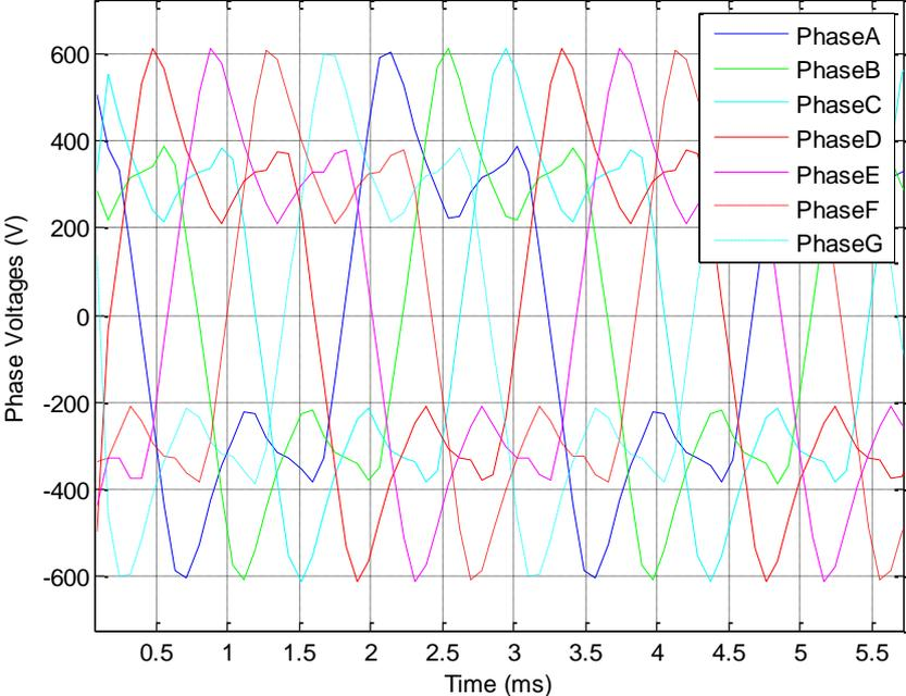
Figure 9: Induced voltages of the 7-phase WRSM
