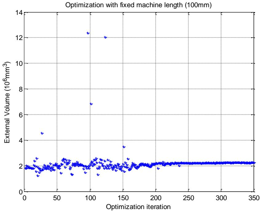
Figure 3. 17: External volume in Optimization with  $L = 100\text{mm}$
