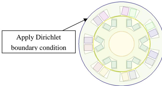
Figure 2. 11: Homogeneous Dirichlet boundary condition
