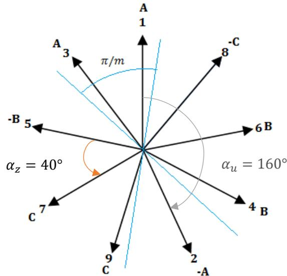
Figure 2. 3: Voltage phasor diagram of 3-phase/9-slot/8-pole machine
