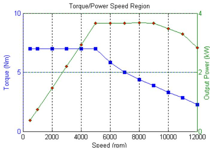
Figure 2. 31: Torque/power vs. speed of the WRSM
