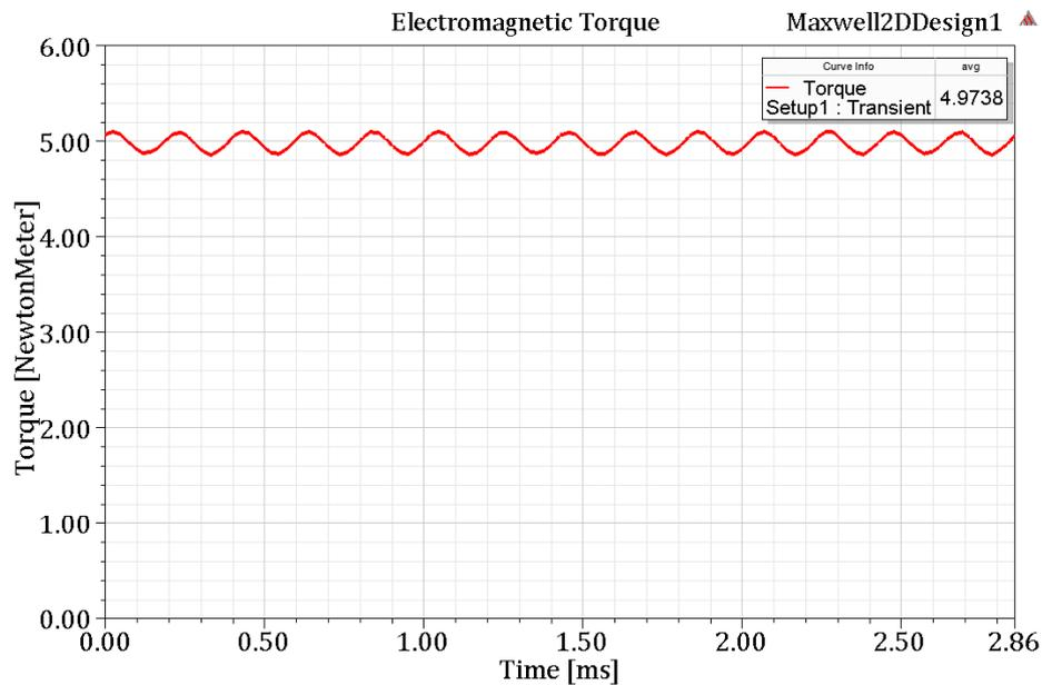
Figure 4. 4: Electromagnetic torque obtained by 2D ANSYS Maxwell 15.1
