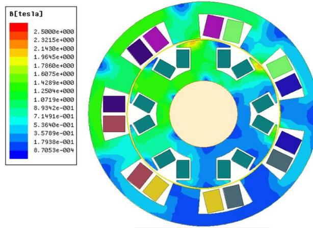
Figure 2. 25: Stator and rotor induction of the WRSM
