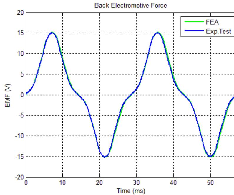
Figure 4. 31: EMF comparison between experimental test and 3D FE analysis
