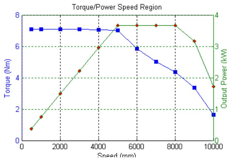
Figure 2.28: Torque and power vs. speed of SM-PMSM
