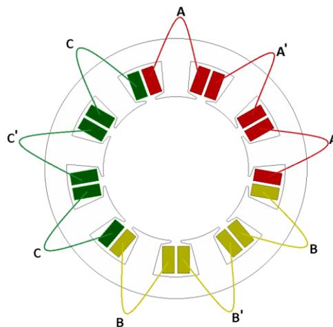
Figure 2. 4: Winding layout of 3-phase/9-slot/8-pole machine
