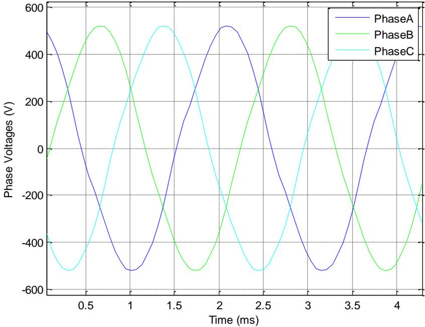
Figure 3: Induced voltage of three phases of SM-PMSM
