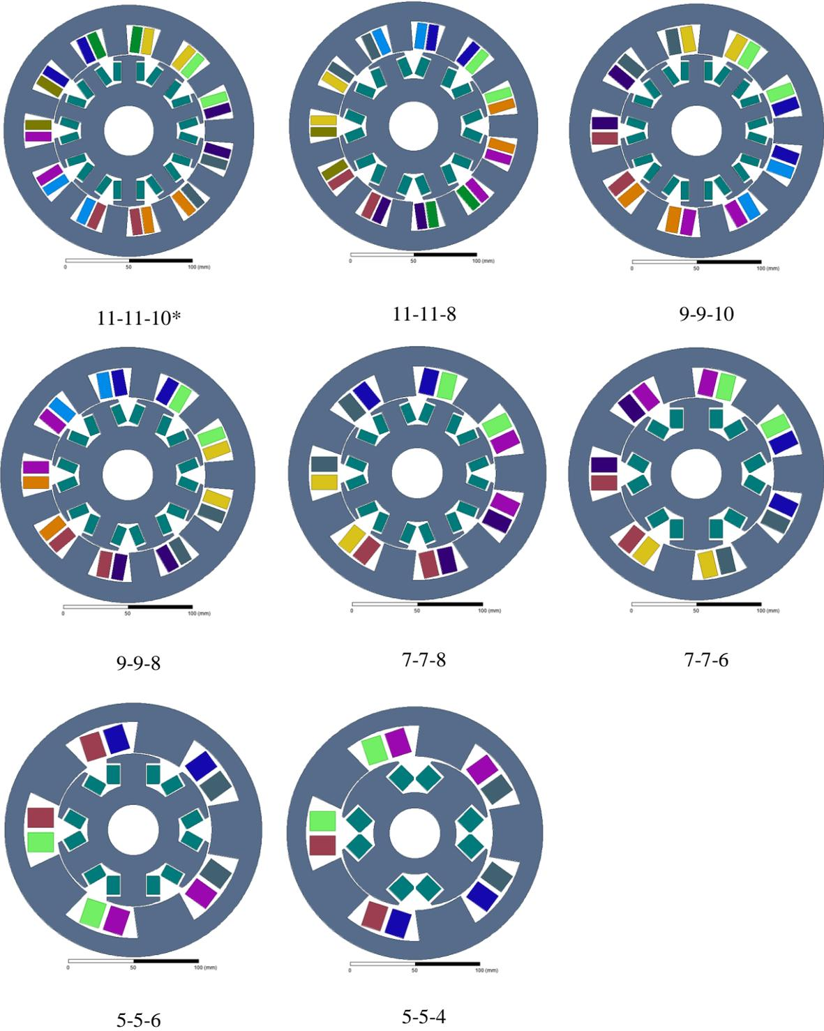
Figure 2. 15: Configurations of studied machines (\* phase-slot-pole number)
