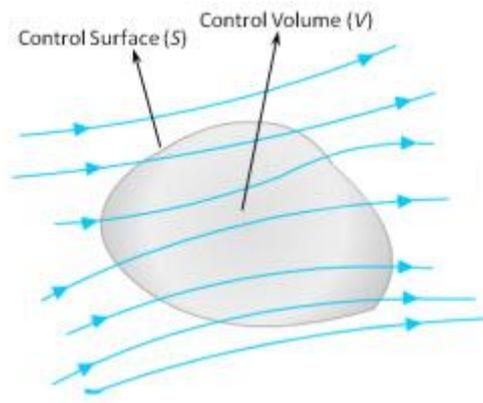
Figure 4. 7: A closed volume within a finite region of flow [113]
