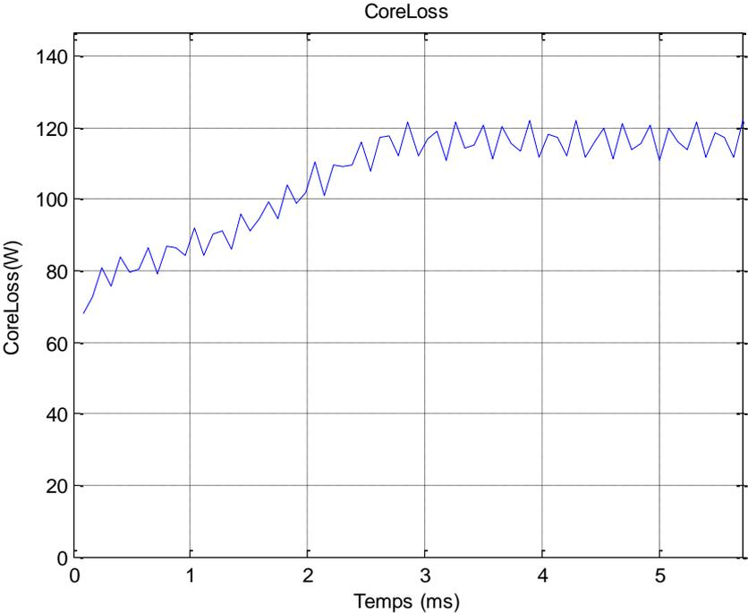
Figure 11: Core losses of the designed WRSM
