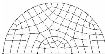
Figure 4. 10: Unstructured grid [15]
