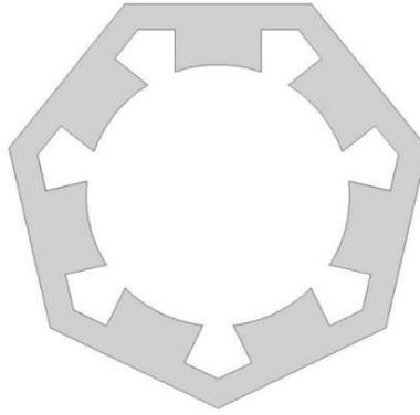
Figure 3. 5: Heptagonal stator of the WRSM
