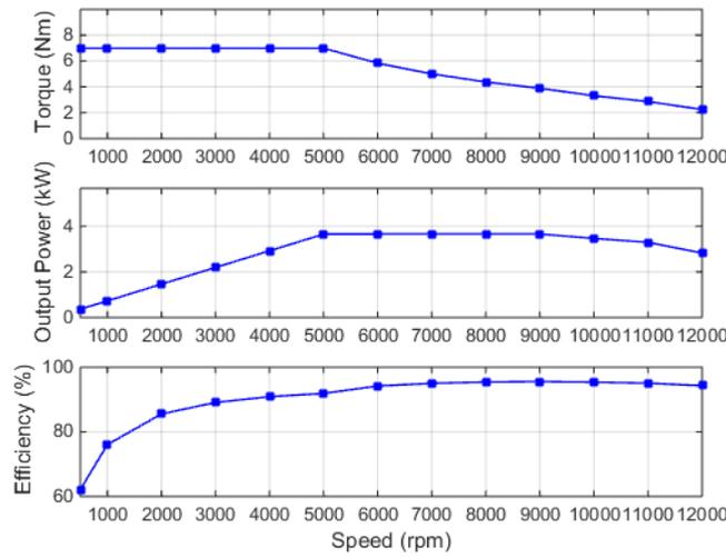
Figure 2. 30: Torque, power and efficiency of the WRSM
