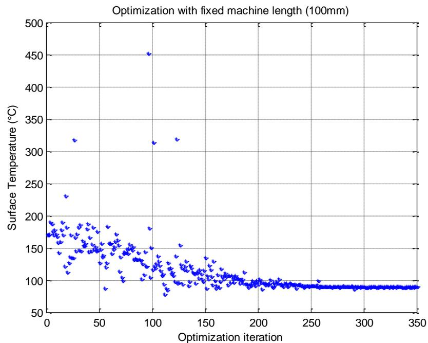
Figure 3. 16: Surface temperature in Optimization with  $L = 100\text{mm}$
