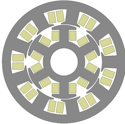
Figure 1. 7: Example of a wound rotor synchronous machine
