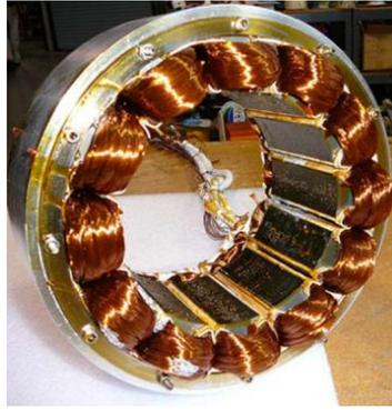
Figure 2. 2: An example of double layer concentrated winding [64]
