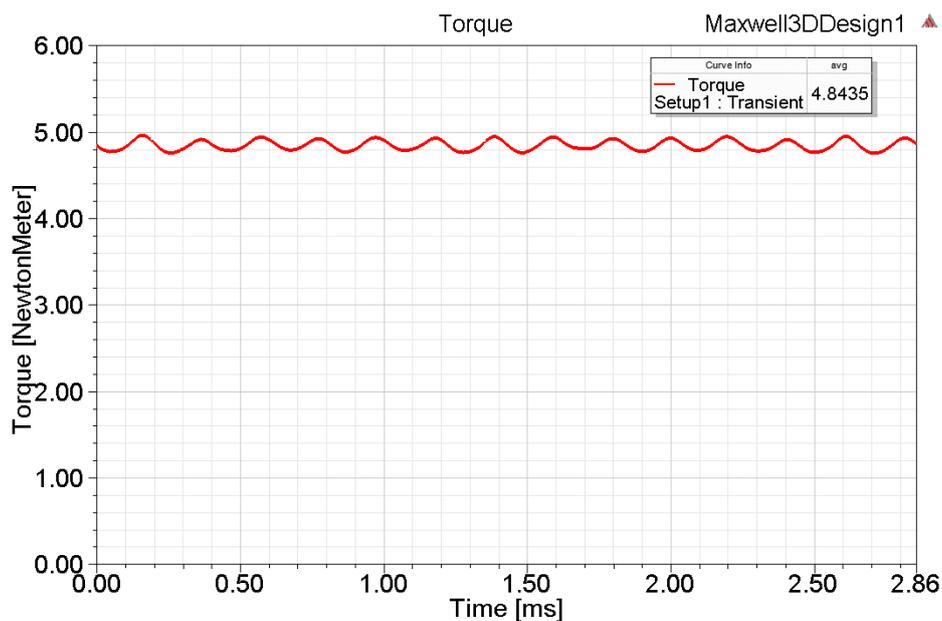
Figure 4. 5: Electromagnetic torque analyzed by 3D ANSYS Maxwell 15.1
