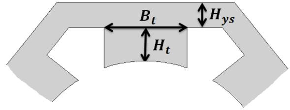
Figure 3. 2: The heptagonal stator variables
