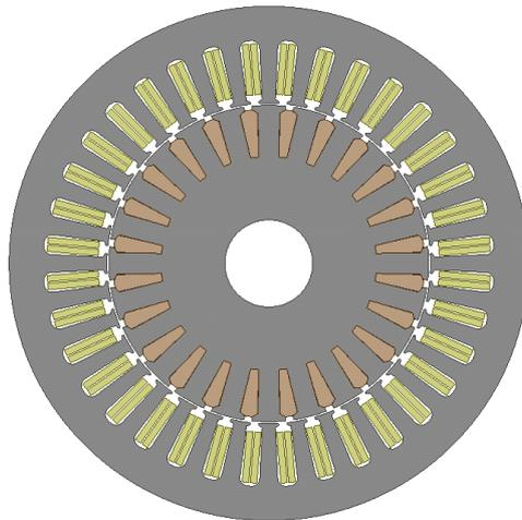
Figure 1. 4: Example of a squirrel cage induction machine
