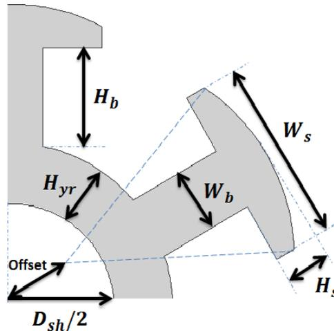
Figure 3. 3: The geometrical variables of the rotor
