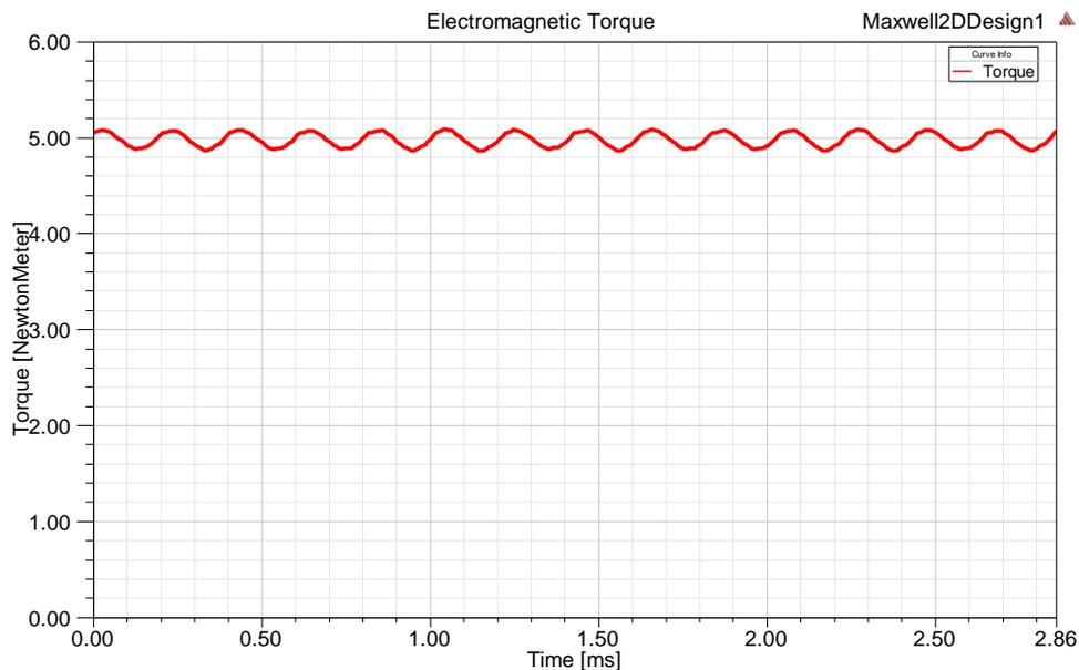
Figure 3. 12: Electromagnetic torque of the optimal WRSM
