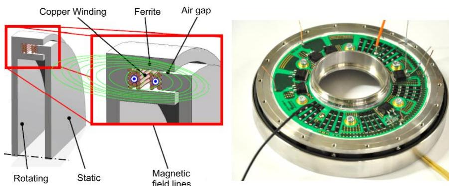
Figure 1. 9: Rotating transformer [35]
