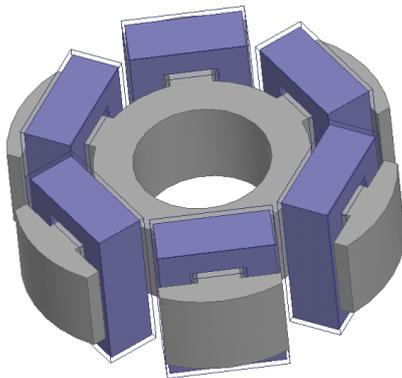
Figure 4. 13: Rotor modelling
