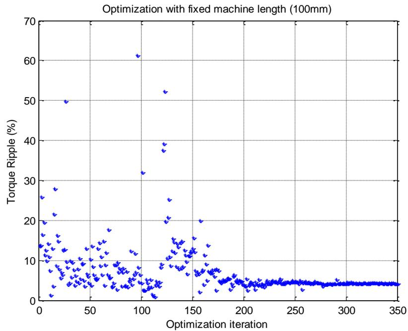
Figure 3. 15: Torque ripple in Optimization with  $L = 100\text{mm}$
