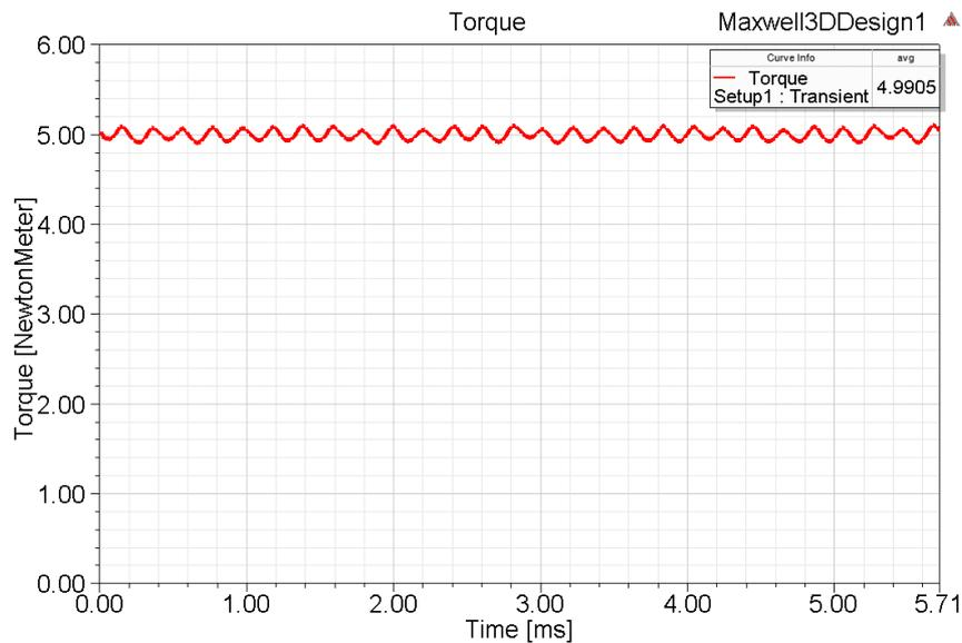
Figure 4. 27: 3D electromagnetic torque of the prototype
