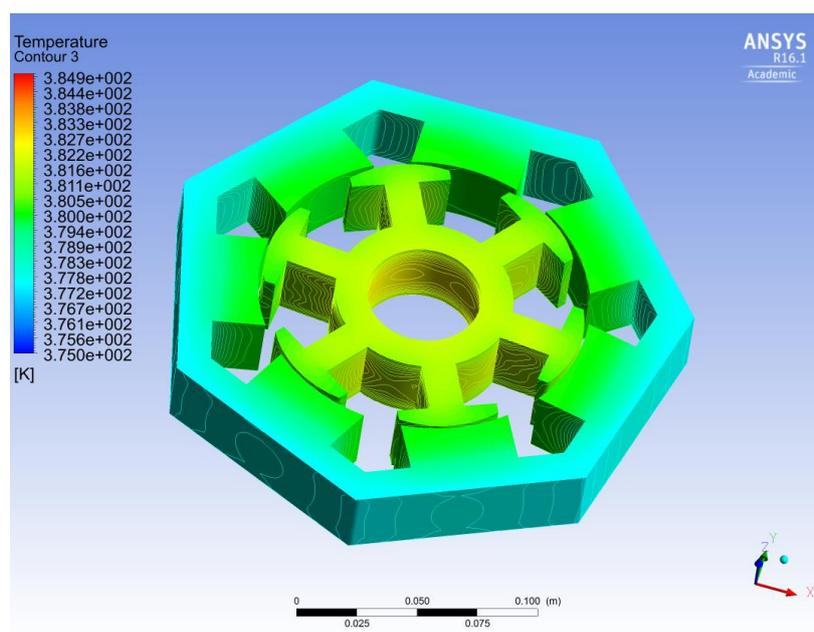
Figure 4. 20: 'zoom' on the temperatures of the laminations
