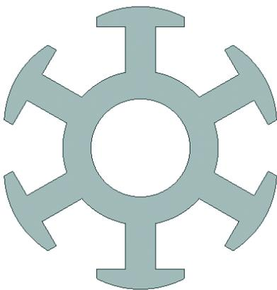
Figure 2. 21: WRSM rotor in 2D
