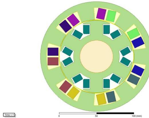
Figure 2. 9: Salient pole wound rotor synchronous machine
