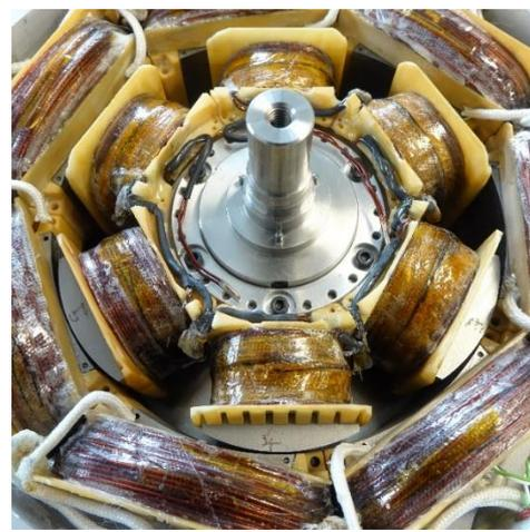
Figure 4. 26: Winding and insulation
