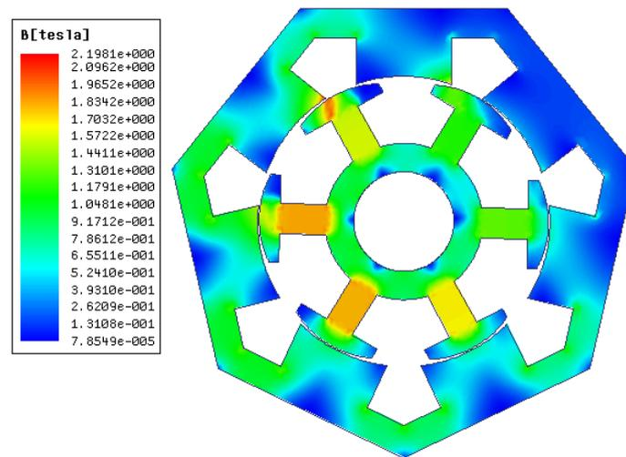
Figure 3. 9: Magnetic induction of the optimal WRSM
