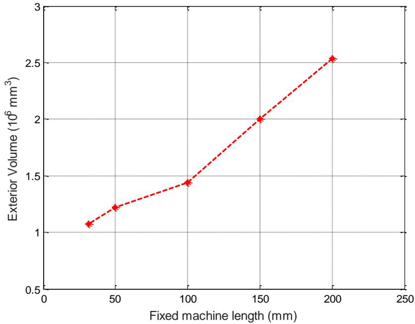
Figure 3. 13: Optimal external volume with fixed machine length
