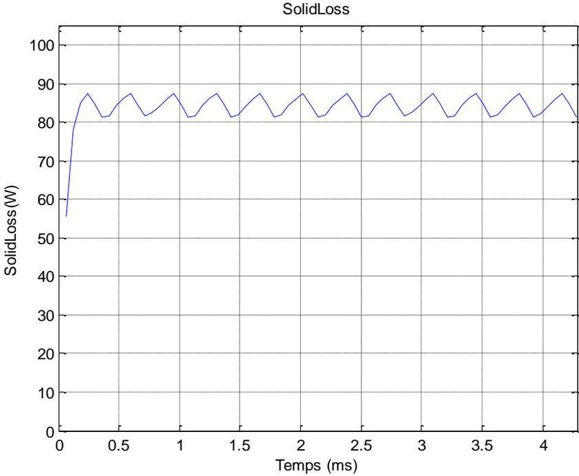
Figure 6: Eddy current losses in permanent magnets
