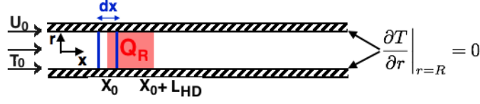
Figure 5.17 Simplified domain: Cylindrical duct with adiabatic walls.
