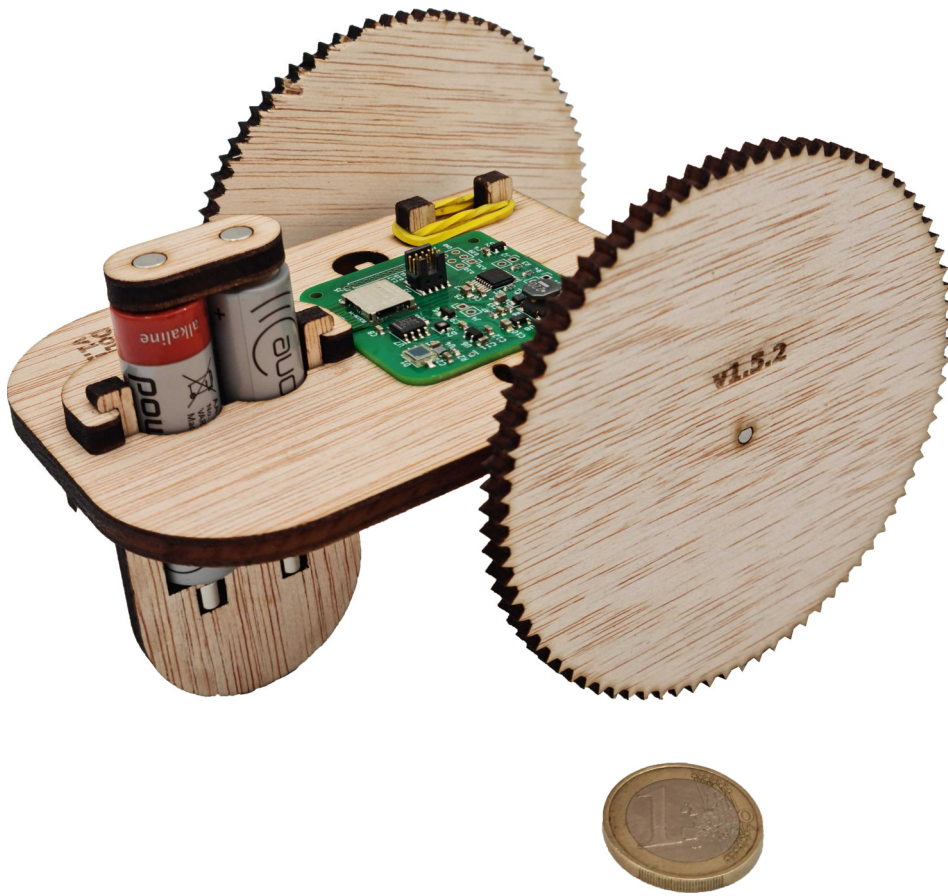
Figure 1.5: DotBot: a low-cost micro-robot for education and research on networking and swarm robotics.
