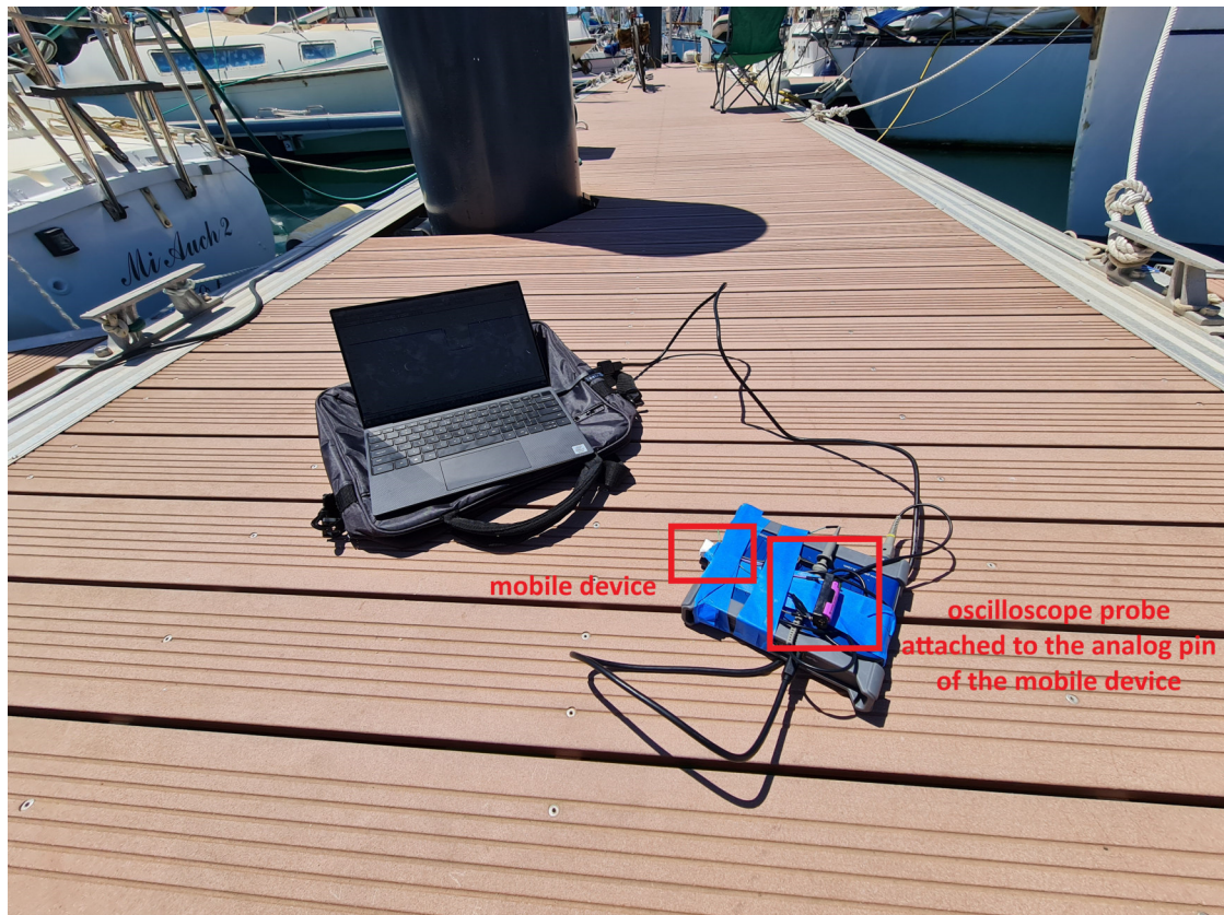
Figure 5.6: Experimental setup for ultrasound detection. We monitor the analog output pin of the mobile device to register an ultrasound signal reception.
