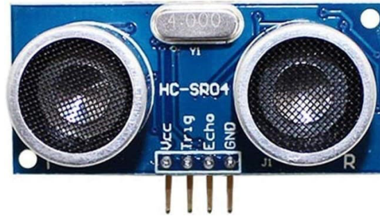
Figure 3.9: The HC-SR04 is ubiquitous in robotic platforms to measure distance to obstacles. It is very easy to find and very cheap. RRDV re-uses it to detect encounters between robots. Note that the CWL-1601 is an equivalent sensor, operating at 3.3 V.
