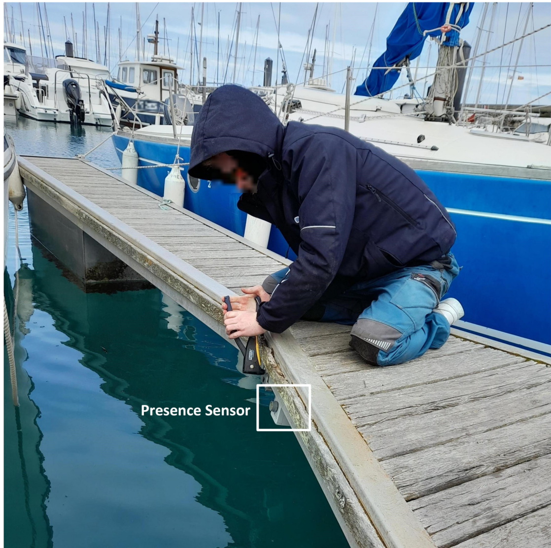
Figure 3.8: Presence sensor for boat detection inside a smart marina.
