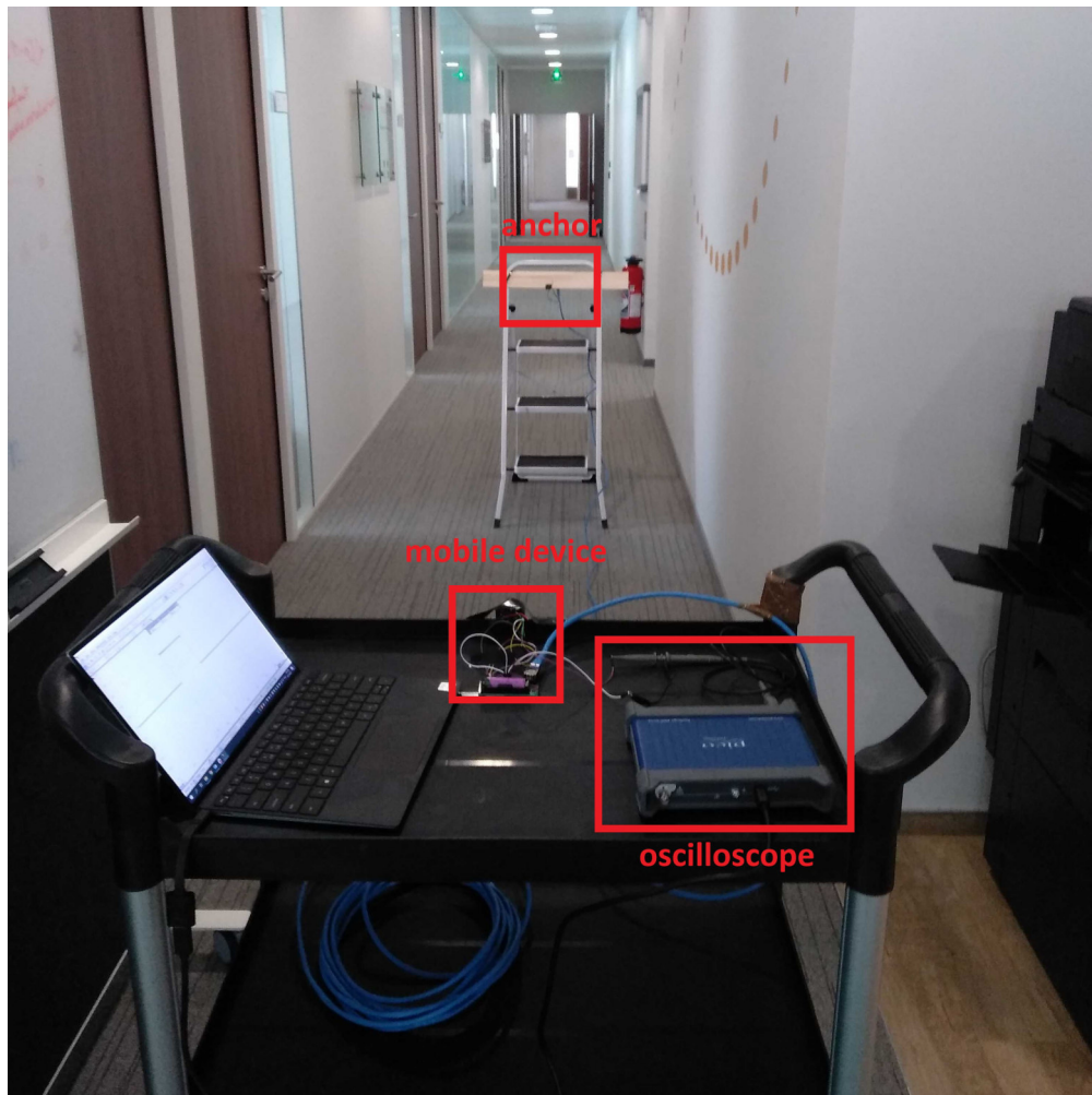
Figure 5.4: Ultrasound ranging test setup located in the corridor of the research laboratory.
