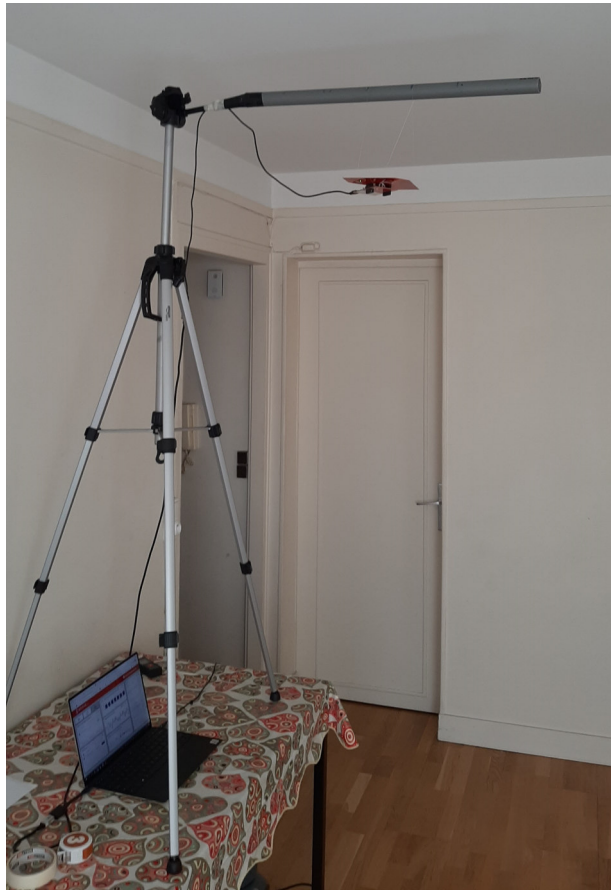
Figure 4.1: BOOSTXL-AOA angle of arrival estimation test setup.
