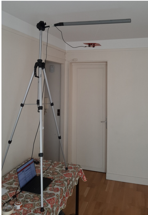
Figure 4.1: BOOSTXL-AOA angle of arrival estimation test setup.
