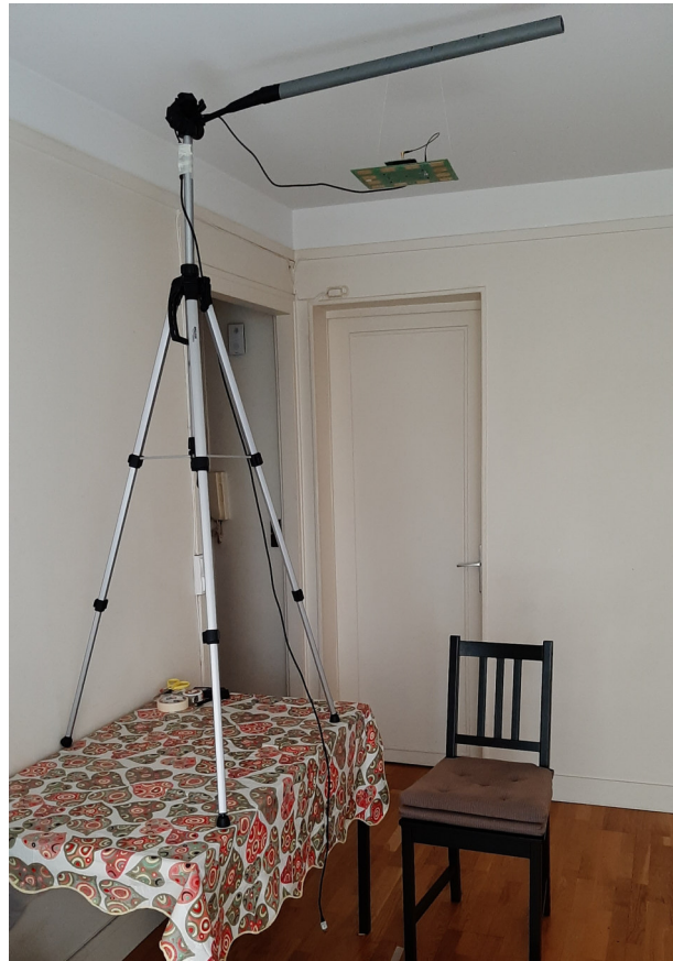
Figure 4.4: Nordic Semiconductor angle of arrival estimation test setup.
