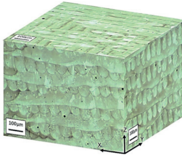
Figure 2.4: Assembly of three perpendicular optical metallographic images of as-built IN718 from [16].
