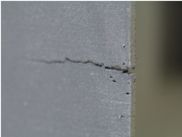
(a) Crack on thin Ti-6Al-4V wall from [60].
