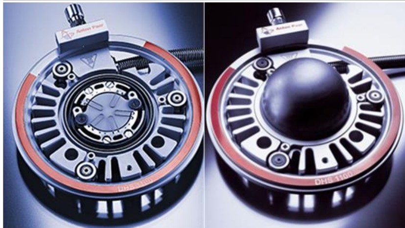
Figure 27 : (a) A Bruker D8 diffractometer in the goniometer configuration and (b) temperature control stage with and without the graphite dome that is used to provide an inert gas atmosphere.
