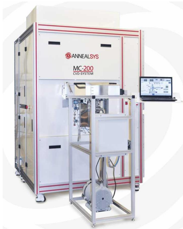
Figure 16 Photograph of the Annealsys MC200 MOCVD reactor at LIST.
