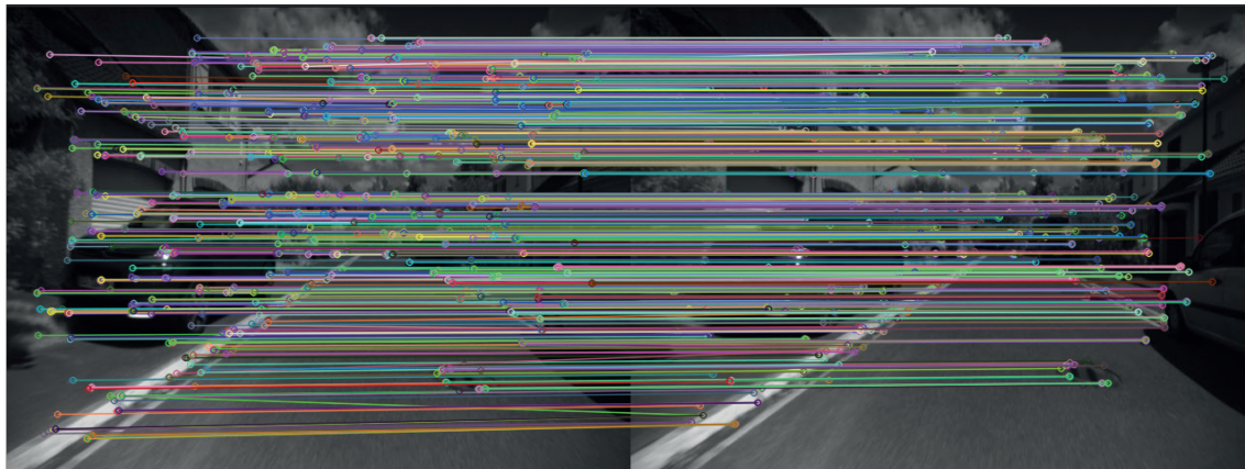
Figure 5.7: Matching two successive images from outdoor sequence 1 on FPGA.
