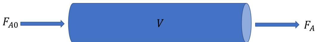
Figure 54: Basic operation mechanism of a plug flow reactor
