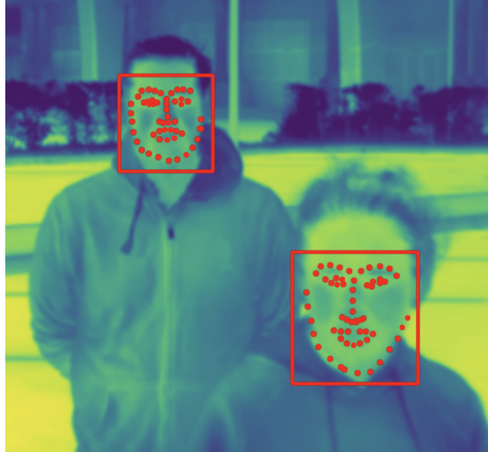
FIGURE 4.12: Examples of TFLD operating in an outdoor environment with sunny weather. Despite challenging atmospheric conditions, faces, eyes, eyebrows, nose, mouth and jawline key points are successfully located by our model (image from TFW [87] dataset).
