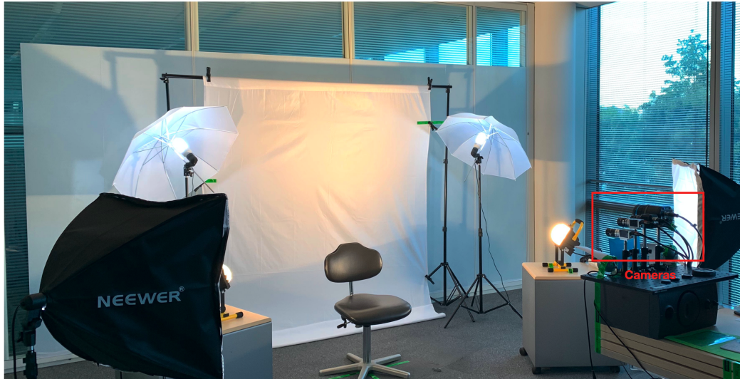
FIGURE 3.2: A glimpse into the acquisition area setup during the BYDB database collection, showcasing the sensor suite (cameras), strategically placed projectors and the thermally neutral white background.
