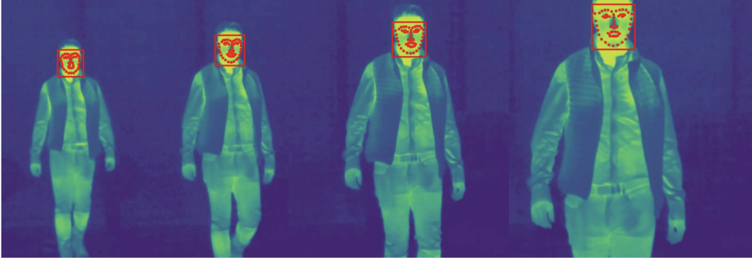
FIGURE 4.1: Monitoring system with thermal sensor. TFLD method applied on video sequence captured in the wild. A person, approximately 14m away, walks towards the camera while TFLD is tracking face and landmarks.
