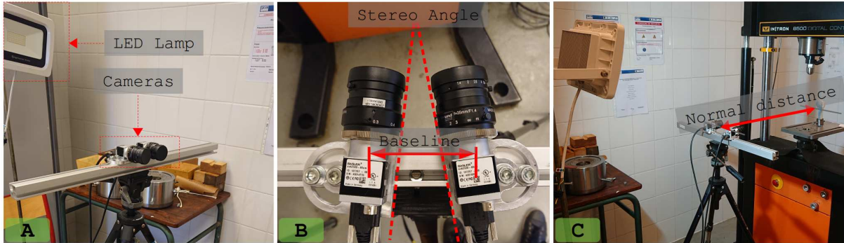
Figure 3.11 – Stereo-rig for the digital image correlation. A: The cameras and the LED lamp. B: The angle used for the cameras ranges between 10° and 20°. C: The normal distance is measured from the baseline to the front of the sample.
