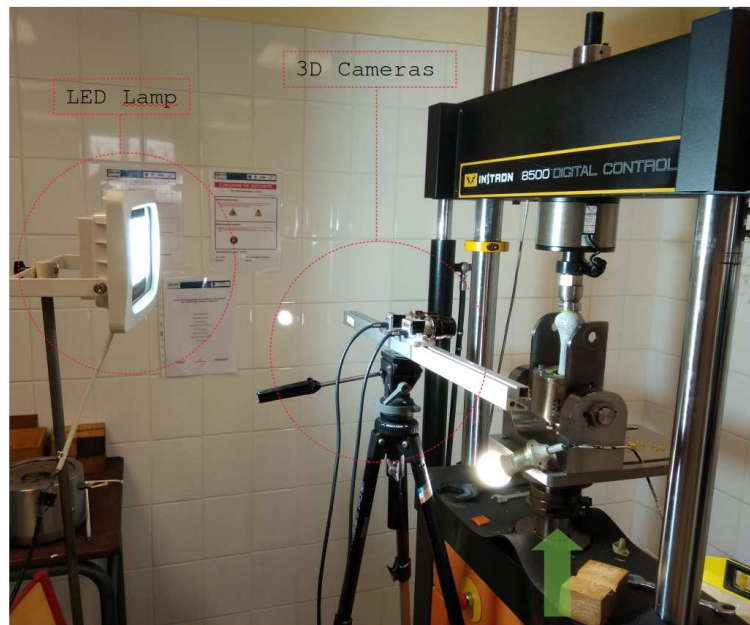
Figure 3.21 – Compression setup at the universal testing machine with the stereo cameras. The green arrow shows the direction of the compressive load.
