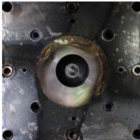
Figure 3.8: Picture of the bottom chamber (R. Lecourt) after tests. The painting has been diluted in the corners by kerosene droplets caught in the recirculation zones (light color).
