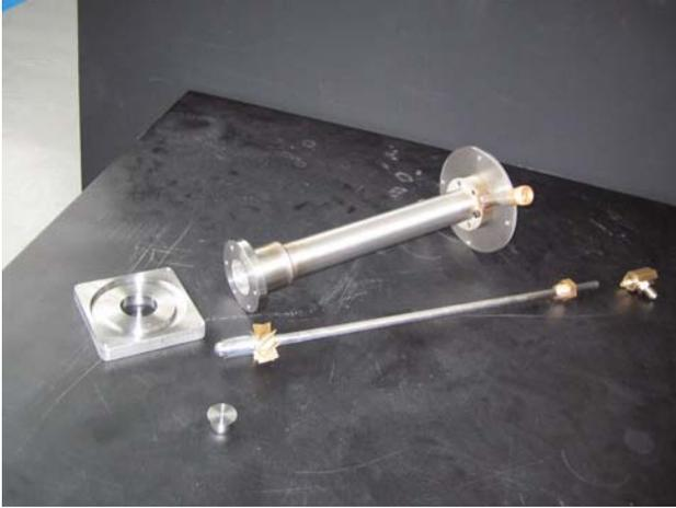
(a) The cylindrical duct bringing the air up to the chamber, the bottom chamber plate and the axial swirler.
