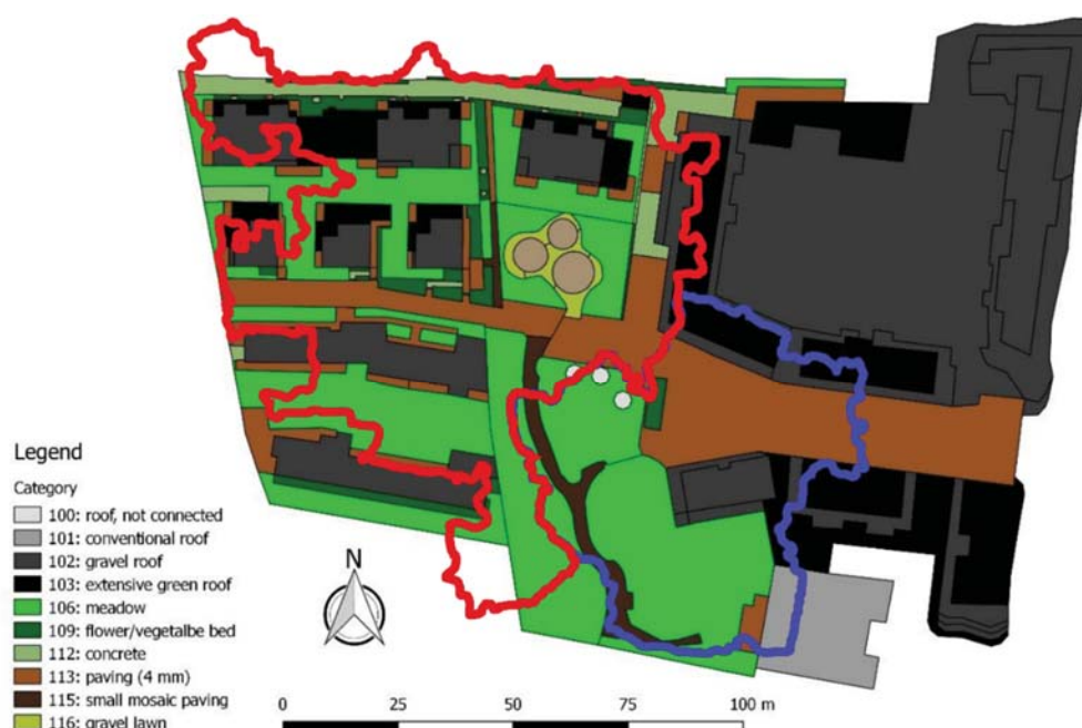
Figure E 3. Categorization of buildings and surface materials and delineation of sub-catchments (sub-catchment trench in red, sub-catchment pond in blue).
