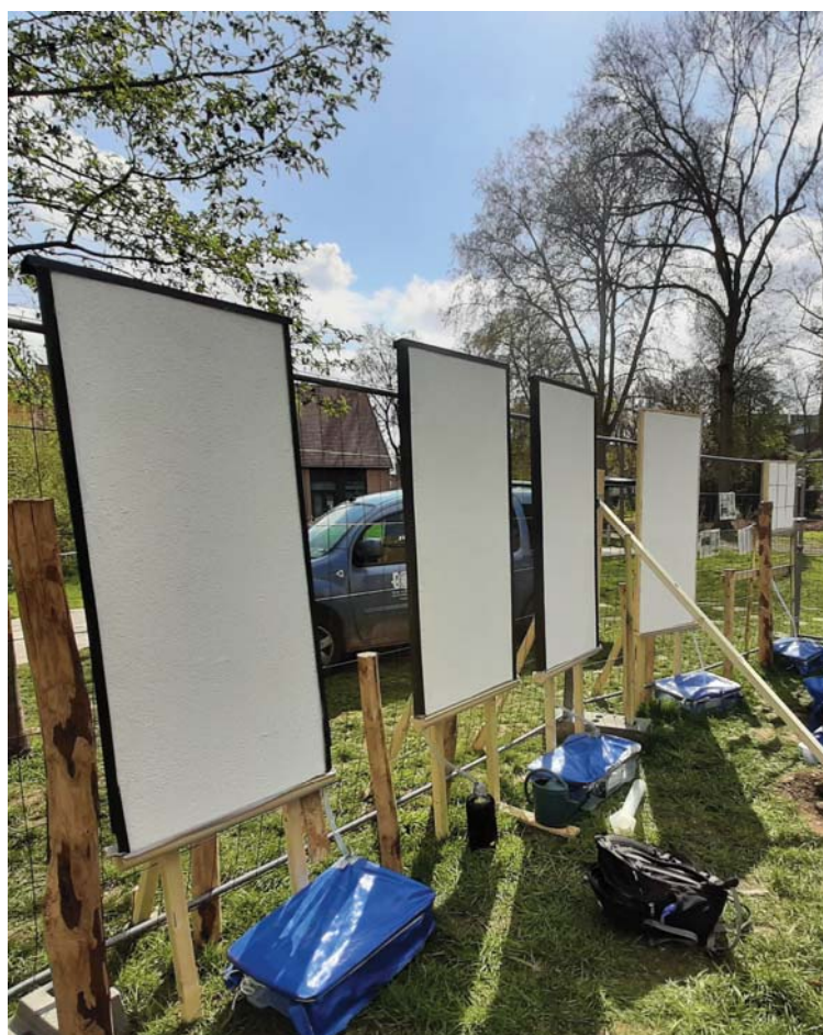
Figure C 1. Experimental setup of facade leaching experiment under environmental conditions.
