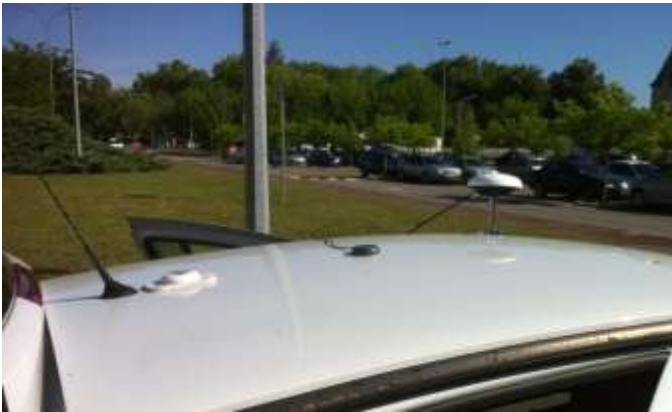
Figure 5.2 Picture of the roof of the car. From left to right: the Novatel L1/L2 patch antenna (in white), the TW2410 patch antenna and the Septentrio L1/L2 geodetic antenna
