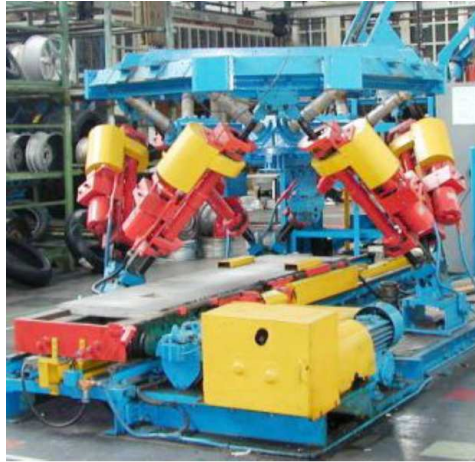
Figure 1.10 – Gough tyre-testing prototype, called universal rig, exhibited in the British National Museum of Science and Industry in 2000 [Bonev, 2003].
