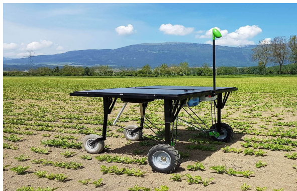
Figure 1.21 – View of ecoRobotix smart weeding robot.
