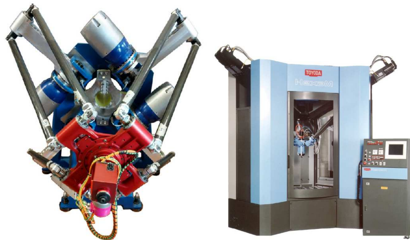
(a) View of SPIDER4 PKM [Escorcía-Hernández et al., 2020b] (b) Toyoda HexaM PKM-based machine tool [Toyama et al., 1998]
