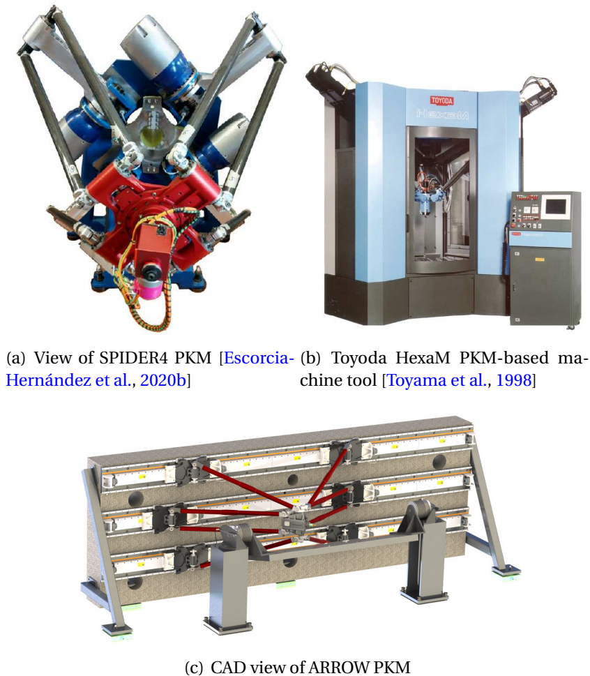
Figure 1.17 – Illustration of three examples of PKMs for machining operations.
