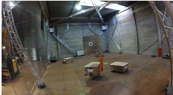
Figure 1.3 – Illustration of the CoGiRo (Control of Giant Robots) prototype built in the framework of a collaborative research project between TECNALIA and LIRMM.
