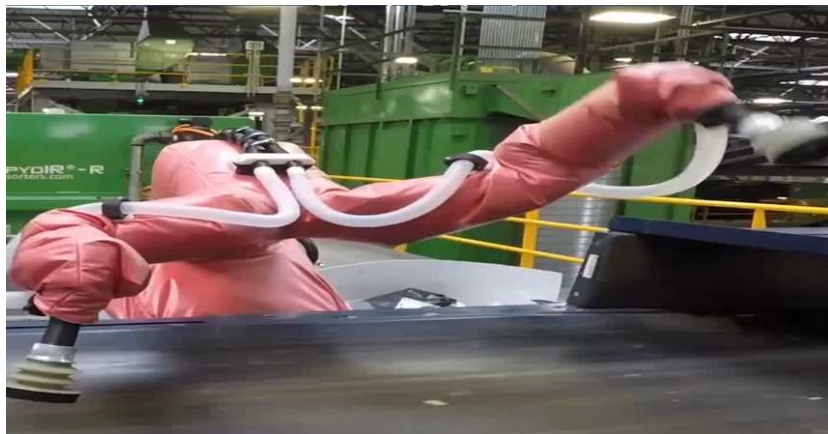
Figure 1.25 – A dual-arm robot uses pick-and-throw in selective waste sorting. This robot was built by "Bulk Handling Systems" to make recycling more efficient.
