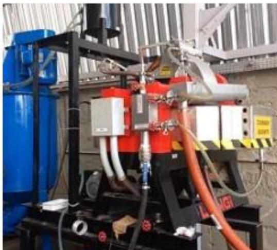
Figure 5. VPHGMS LGS-EX adopted in the exploratory pilot tests to evaluate the magnetic concentration of iron ore slimes from the Vargem Grande 2 plant.
