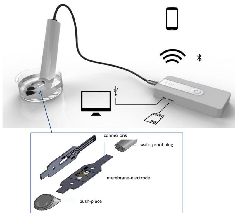
**Fig. 10.** Photograph of the prototype showing, immersed in a 125 mL glass beaker container, a support holding the membrane-electrode pad. Membrane-electrode pads are connected to the measurement device via the support cable -inset: pad components, the membrane-electrode is sandwiched in middle where the open windows allow a permanent contact with the electrolyte. A dedicated software drives the overall system.
