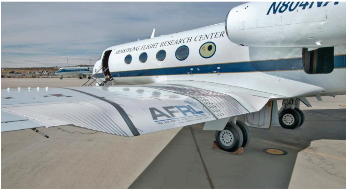
Figure 1.5: Picture of the Gulfstream III Subsonic Research Aircraft Testbed, with the morphing flap prototype from [Mil+16]
