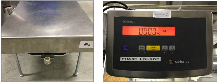
Fig.3. 24 - Sartorius Combics 1 CAW1P*L precision balances
