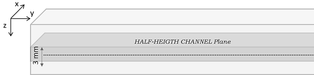
Fig.3. 11 – PIV measurement plane in z-direction
