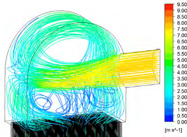
Fig.5. 34 - Velocity streamlines at the inlet header for \alpha = 0^\circ
