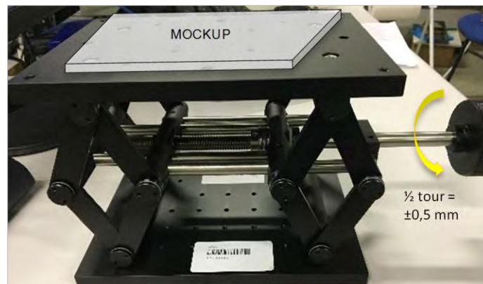
Fig.3. 17 – Mockup displacement device
