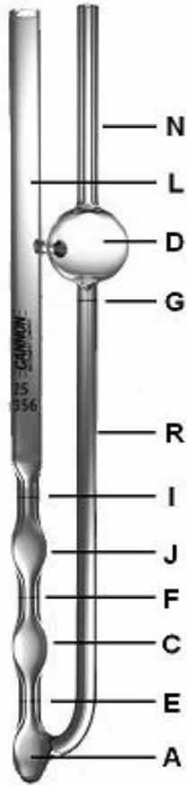
Fig. 1. The Cannon-Fenske opaque viscometer
