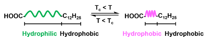
Scheme IV.6 Structure and effect of temperature on the conformation of PN chains at pH 4.
