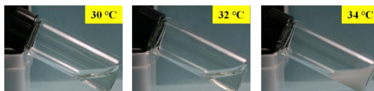
Figure III.24 Photographs of phase states of PBA 2k - b -PNIPAM 8k (5 wt.% in water) at 30, 32 and 34 °C (The sample was equilibrated in a dry box for 5 min at a given temperature before visual observation, then the same procedure was operated at higher temperature after sample recovered to transparent state).
