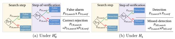
Figure 3.16 Probabilities per cell at the output of the acquisition step
