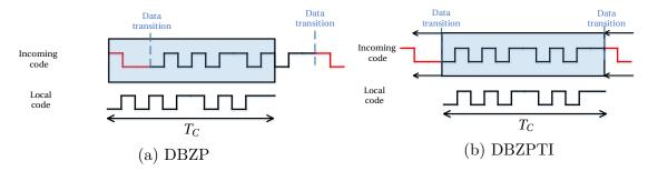
Figure 5.12 Transition insensitivity of the DBZPTI
