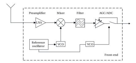
Figure 2.6 Illustration of an RF front-end
