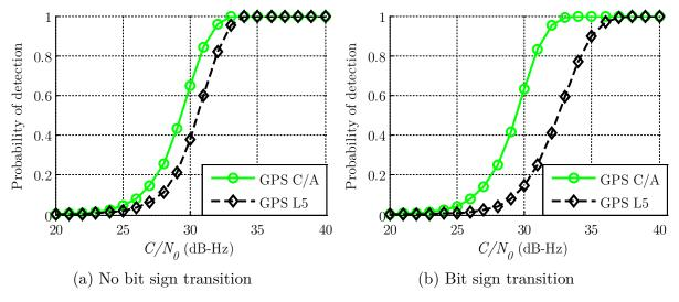
Figure 4.32 Probabilities of detection when considering or not bit sign transitions on  $T_I = 20$  ms and  $T_C = 1$  ms for GPS L1 C/A and GPS L5
