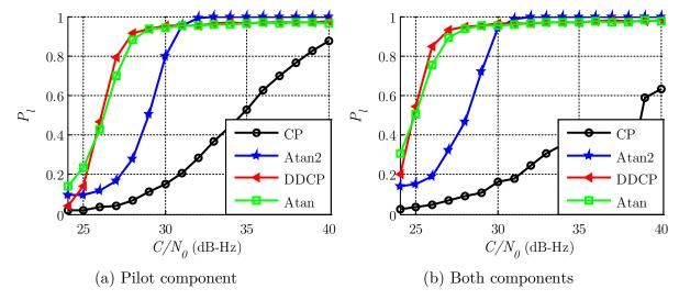
Figure 7.20 Results for FLL schemes for Galileo E1 OS with a frequency update every 8 ms ( $C/N_0 = 27$  dB-Hz,  $T_C = 4$  ms)
