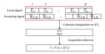
Figure 4.13 Coherent summation scheme when considering code Doppler on the received signal
