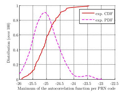
Figure C.6 Distribution of the maximum Galileo PRN codes autocorrelation function per PRN code (excluding the correct code delay alignment)
