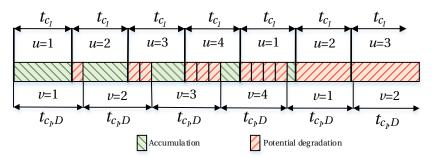
Figure 4.5 Autocorrelation process: same spreading code but with different length due to code Doppler
