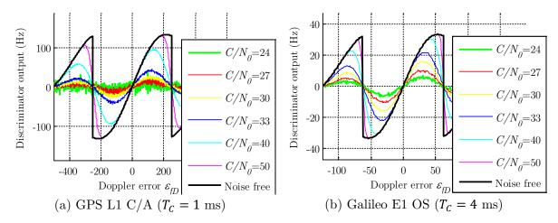
Figure 7.3 DDCP discriminator response to frequency error for a noise-free signal and different  $C/N_0$  cases
