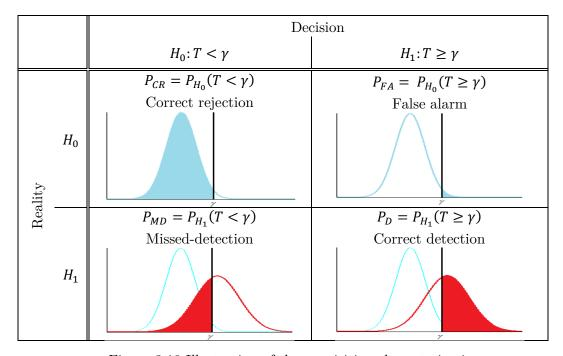
Figure 3.10 Illustration of the acquisition characterization
