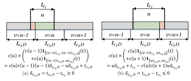
Figure E.1 Product of the chip "u" of the local spreading code by the received spreading code
