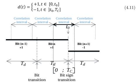
Figure 4.16 Bit sign transition scheme
