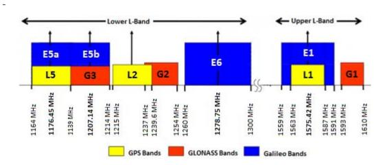
Figure 2.1 GPS, GLONASS and Galileo navigational frequency bands
