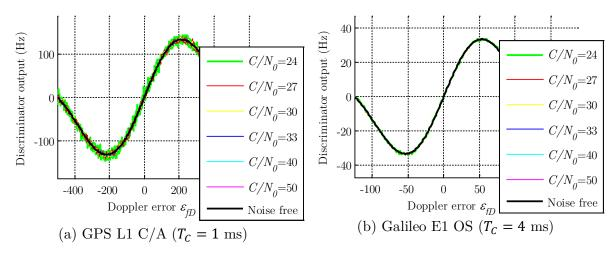
Figure 7.2 Average CP discriminator response to frequency error for a noise-free signal and different  $C/N_0$  cases
