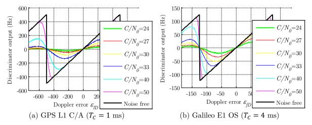
Figure 7.5 Atan2 discriminator response to frequency error for a noise-free signal and different  $C/N_0$  cases
