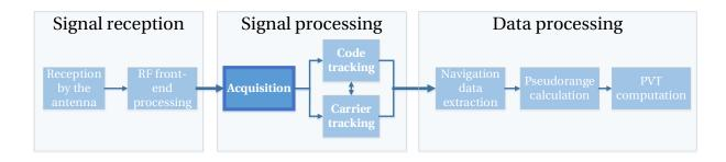
Figure 1.1 General view of a GNSS receiver
