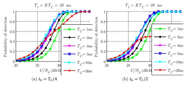
Figure 4.21 Probabilities of detection for different coherent integration times and different location of the transition when considering bit sign transition (GPS L1 C/A)
