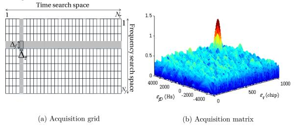
Figure 3.7 Matrix acquisition based on an acquisition grid
