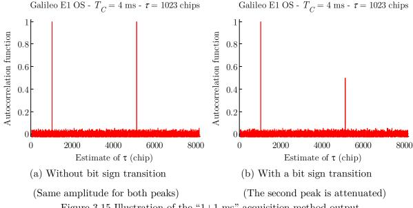
Figure 3.15 Illustration of the "1+1 ms" acquisition method output
