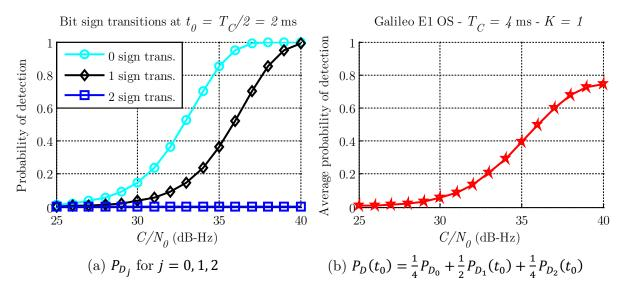
Figure 4.25 Probabilities of detection  $P_{Dj}$  and  $P_D(t_0)$  for one integration (K = 1) on 4 ms on both components and considering a bit sign transition in the middle of the integration interval (Galileo E1 OS)
