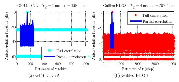
Figure 5.3 Full and partial GPS L1 C/A and Galileo E1 OS autocorrelations
