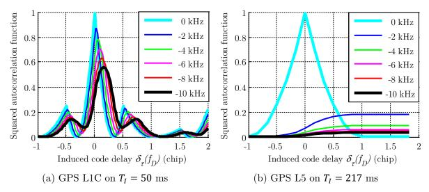
Figure 4.9 Normalized squared autocorrelation function when considering code Doppler
