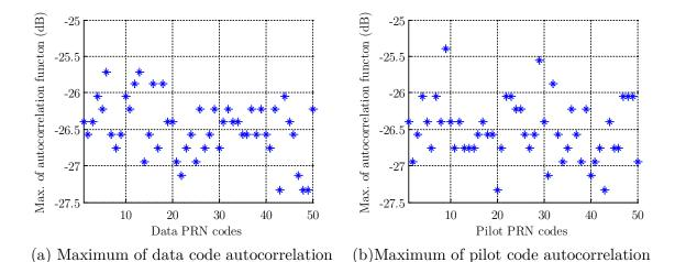
Figure C.5 Maximum of the autocorrelation function per PRN code (excluding the correct code delay alignment and no Doppler)
