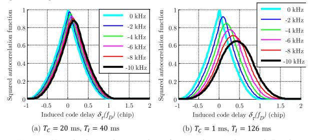
Figure 4.7 Normalized squared autocorrelation function when considering code Doppler (GPS L1 C/A)
