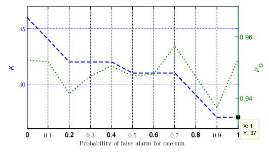
Figure 6.5 Required number of non-coherent summations for Approach 3
