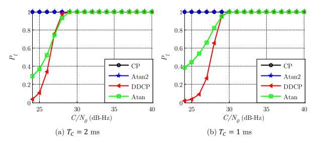
Figure 7.23 Results for FLL schemes for Galileo E1 OS with a frequency update every 20 ms (both components)
