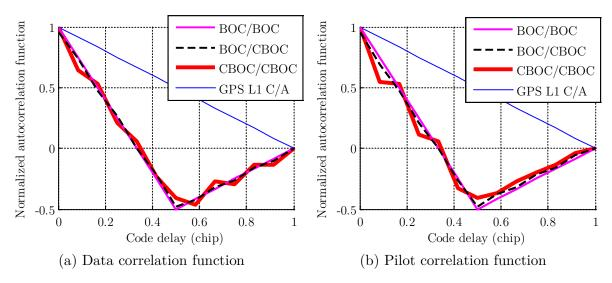
Figure 2.5 Normalized correlation function shapes of Galileo and GPS L1  $\rm C/A$  spreading codes (as a function of the modulation)
