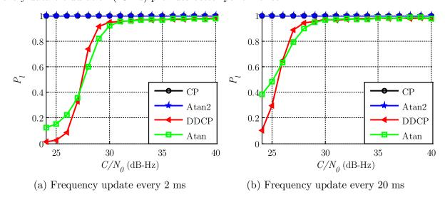
Figure 7.18 Results for FLL schemes for GPS L1 C/A
