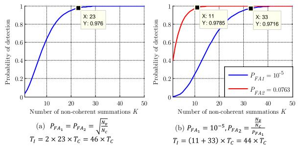
Figure 6.4 Examples of acquisition performance for 2 choices of probabilities of false alarm for Approach 3 ( $C/N_0 = 27$  dB-Hz)
