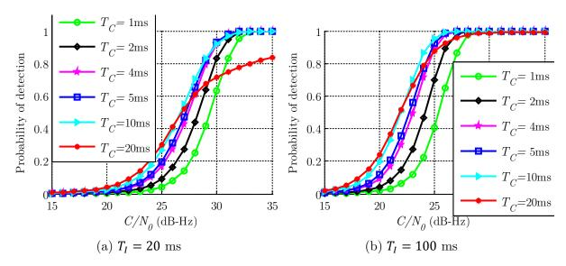
Figure 4.23 Average probabilities of detection on  $t_{\theta}$  for different coherent integration times when considering bit sign transition (GPS L1 C/A)
