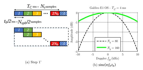
Figure 5.13 Losses reduction due to high Doppler frequencies
