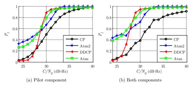
Figure 7.30 Results for FLL schemes for Galileo E5 with a frequency update every 20 ms ( $T_C = 1 \text{ ms}$ )
