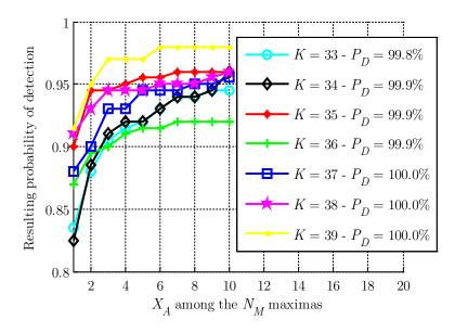
Figure 6.3 Required number of non-coherent summations for the Approach 2  $(C/N_0 = 27 \text{ dB-Hz})$
