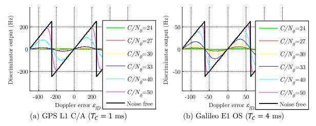
Figure 7.4 Atan discriminator response to frequency error for a noise-free signal and different  $C/N_0$  cases
