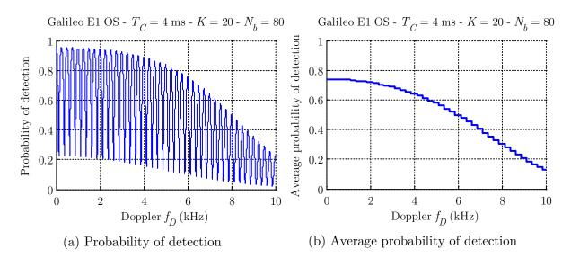
Figure 5.10 Probability of detection as a function of the incoming Doppler frequency for the DBZP acquisition method (no code delay error)
