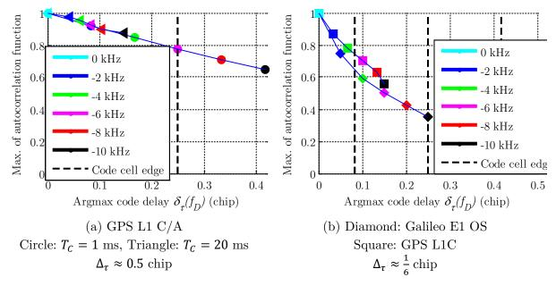
Figure 4.10 Description of the peak (amplitude and argmax) of the autocorrelation function
