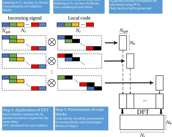
Figure 5.6 Double-Block Zero-Padding (DBZP) method block diagram
