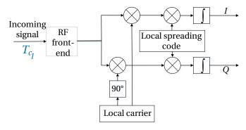
Figure 3.2 Block diagram of the correlation
