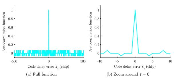
Figure 3.1 GPS L1 C/A autocorrelation function (PRN 2)
