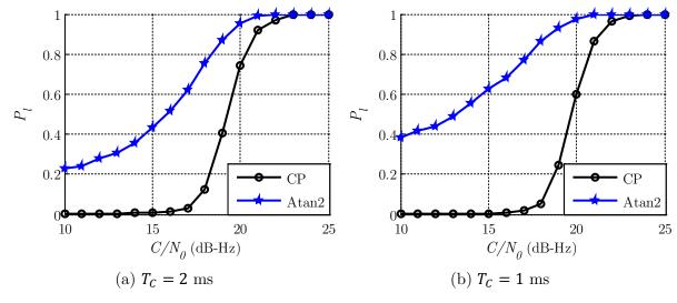
Figure 7.24 Results for FLL schemes for Galileo E1 OS with a frequency update every 20 ms (both components) (low  $C/N_0$ )
