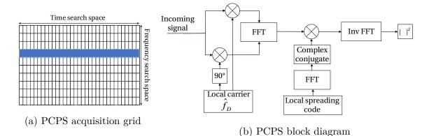
Figure 3.13 Block diagram of the PCPS
