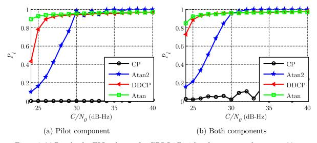
Figure 7.26 Results for FLL schemes for GPS L1C with a frequency update every 20 ms ( $T_C = 10 \text{ ms}$ )
