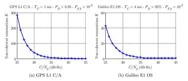
Figure 6.7 Required number of non-coherent summations as a function of the  $C/N_0$  (DBZPTI method, no errors, null incoming Doppler frequency)
