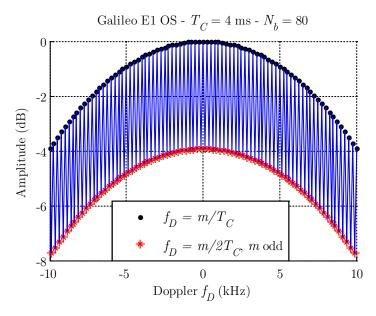
Figure 5.9 Losses due to the incoming Doppler frequency
