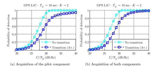
Figure 4.30 Probabilities of detection on  $T_I = 20$  ms when considering or not bit sign transitions (GPS L1C)
