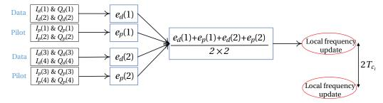
Figure 7.13 FLL technique applied to data/pilot GNSS signals using partial correlations. As previously, a variant of this technique consists in updating every 20 ms instead of  $2T_{c_1}$ .
