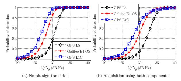
Figure 4.31 Probabilities of detection for  $T_I = 20$  ms when considering or not bit sign transitions (modernized GNSS signals)
