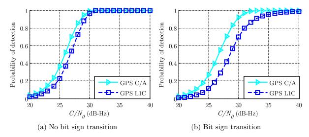
Figure 4.34 Probabilities of detection when considering or not bit sign transitions on  $T_I = 20 \text{ ms}$  and  $T_C = 10 \text{ ms}$  for GPS L1 C/A and GPS L1C
