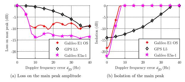
Figure 7.40 Pilot secondary code correlation properties in presence of residual Doppler frequency error
