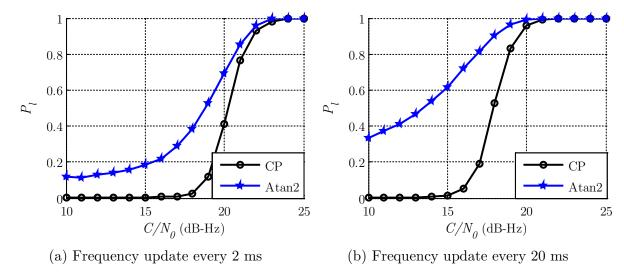
Figure 7.19 Results for FLL schemes for GPS L1 C/A (low  $C/N_0$ )
