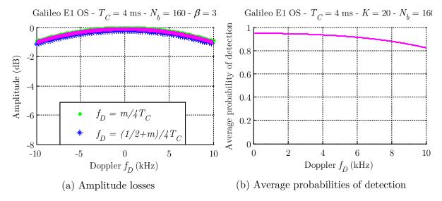
Figure 5.15 Losses due to the incoming Doppler frequency after improvements
