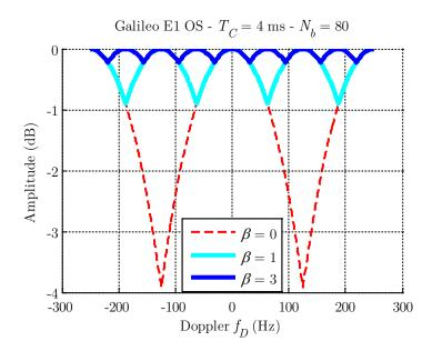
Figure 5.14 Losses reduction at intermediate incoming Doppler frequencies
