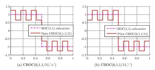
Figure 2.3 Galileo E1 OS CBOC(6,1,1/11) subcarriers modulating one PRN chip
