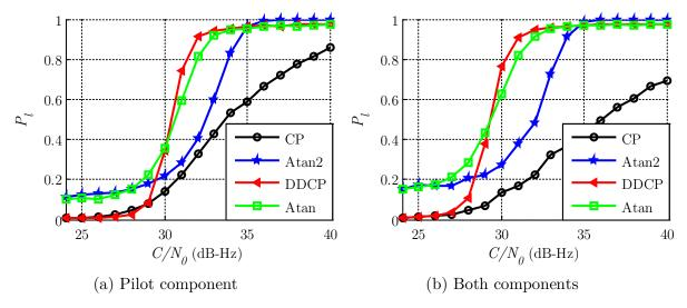
Figure 7.29 Results for FLL schemes for Galileo E5 with a frequency update every 2 ms ( $T_C = 1 \text{ ms}$ )
