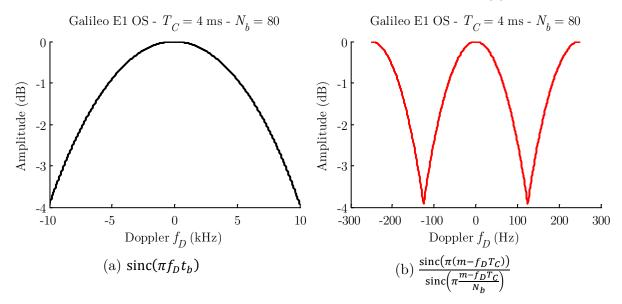
Figure 5.7 Degradations of the criterion due to incoming Doppler frequency
