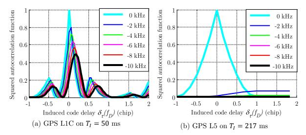
Figure 4.15 Normalized squared autocorrelation function when considering code Doppler (coherent summation – GPS L1C and L5)
