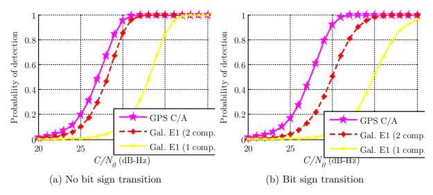
Figure 4.33 Probabilities of detection when considering or not bit sign transitions on  $T_I = 20$  ms and  $T_C = 4$  ms for GPS L1 C/A and Galileo E1 OS
