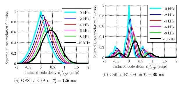
Figure 4.14 Normalized squared autocorrelation function when considering code Doppler (coherent summation – GPS L1 C/A and Galileo E1 OS)
