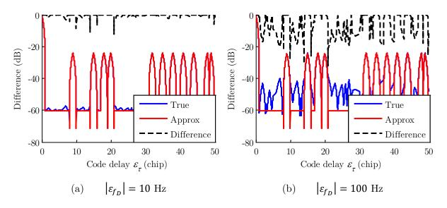
Figure 3.6 Comparison of the CAF of PRN 1 when  $|\varepsilon_{ID}|$  is relatively small
