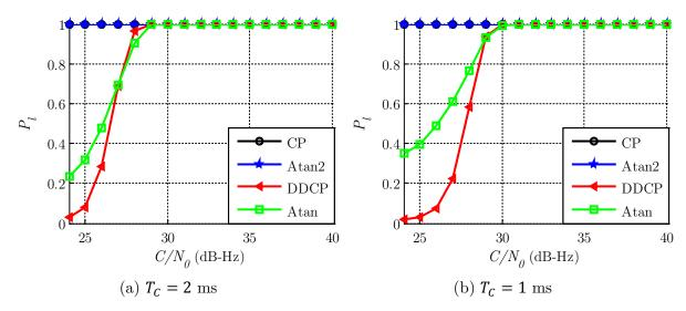
Figure 7.22 Results for FLL schemes for Galileo E1 OS with a frequency update every 8 ms (both components)
