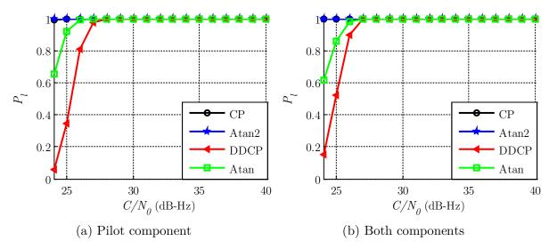
Figure 7.27 Results for FLL schemes for GPS L1C with a frequency update every 20 ms ( $T_C = 5 \text{ ms}$ )
