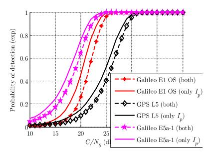
Figure 7.39 Comparison of the secondary code acquisition methods for three signals (K=1)
