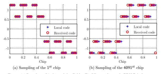
Figure 4.4 Sampling of 2 chips of the Galileo E1 OS spreading code PRN B/1 for an incoming Doppler frequency of 10 kHz and a sampling frequency of 40.96 MHz
