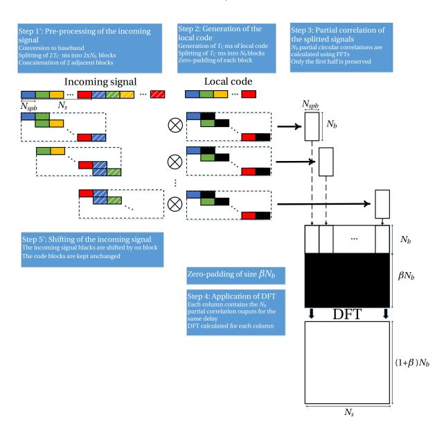
Figure 5.16 DBZPTI method block diagram
