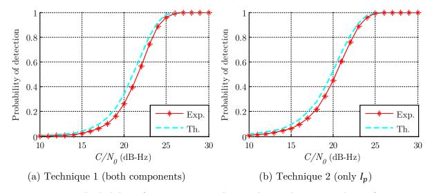
Figure 7.38 Probability of correct main peak secondary code autocorrelation function detection for both techniques (applied to Galileo E1 OS for K = 1)
