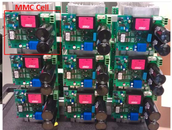
Figure A - 6: Cells on the heatsinks
