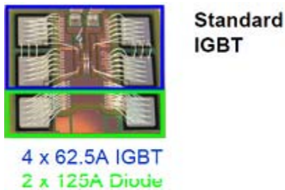
Figure I-24: Multi chip configuration proposed by ABB
